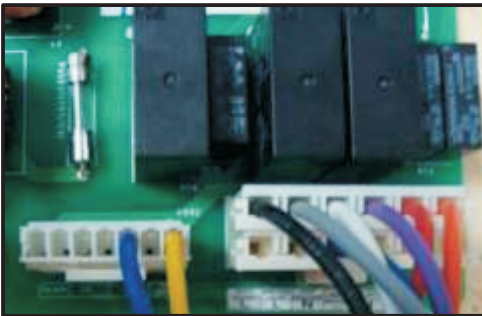
*LOAD DRIVE AREA ON MAIN PCB
