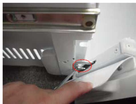
With a small screwdriver, lift lever ② from lever ③ to engage lever ①.
