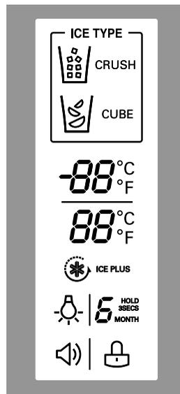
\* LED check function : If simultaneously pressing Ice Plus button and freezing temperature adjustment button for a second, display LED graphics on. If releasing the button, the LED graphic displays the previous status.
