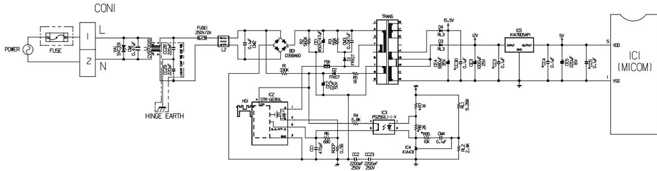
The secondary part of the TRANSFORMER is composed of the power supply for the display, the BLDC FAN Motor drive (15.5V), the relay drive (12 Vdc) and the MICOM and IC (5 Vdc).
