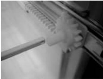
Step 3) Insert the rail into the left side gear, and insert the gear into the clip.
