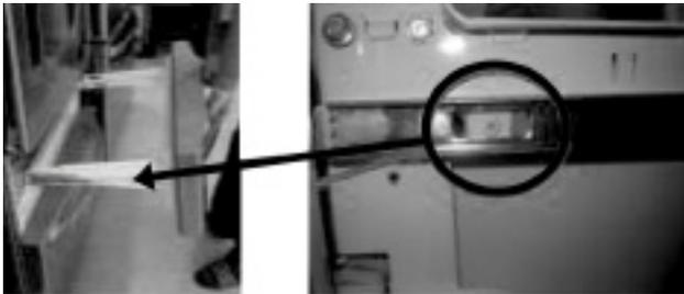
Step 4) Lift the freezer door up to unhook it from the rail support and remove. Pull both rails to full extension.
