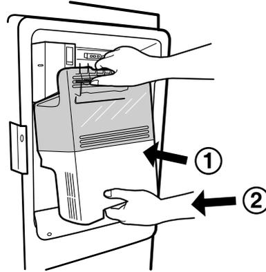
※ Insert the ice bucket carefully avoid contacting the automatic shut off arm.
