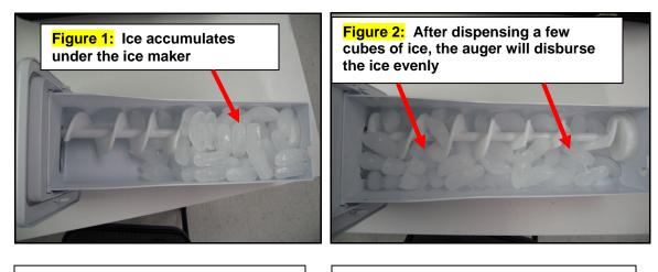
In the initial ice making process, the cubes accumulate at the rear of the ice bucket, under the ice maker as shown above. After the initial ice making process, dispensing a few cubes will allow the auger to disburse the cubes evenly.
