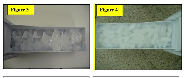
After an additional 6 hours, cubes once again accumulate at the rear of the ice bucket.
