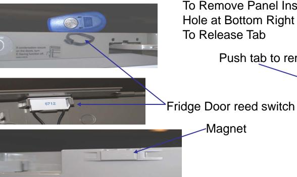
To Remove Panel Insert Small Screwdriver in Square Hole at Bottom Right Corner. Push Screwdriver to Left To Release Tab
