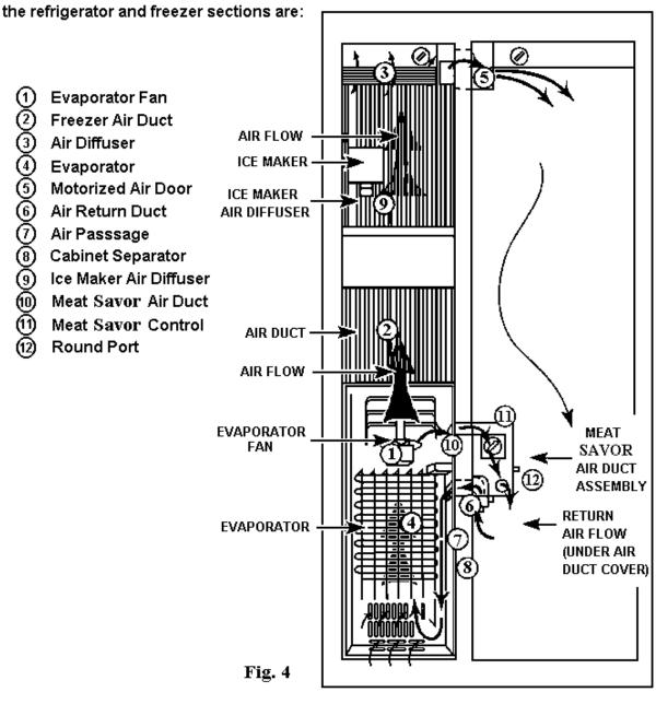
Figure 4 illustrates all of the components used in the circulating air through the freezer and refrigerator compartments.
