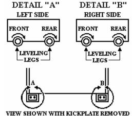
**NOTE:** DO NOT use an electric driving device. Over tightening can cause damage.
