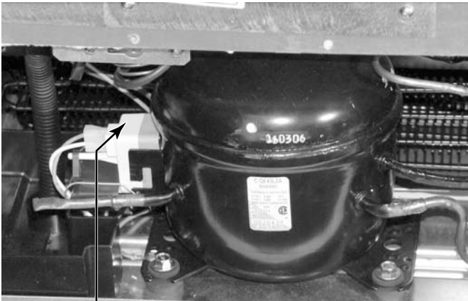
Remove the Run Capacitor and Relay / Overload
