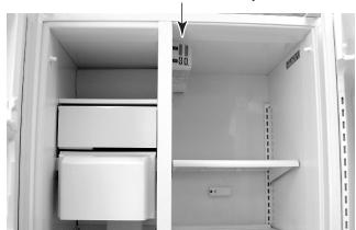
Remove the light shield. To do this, place your finger into the half-moon slot at the bottom of the shield and pull out, then pull down to disengage the corners from the control box.
