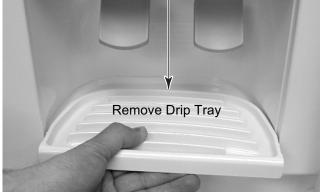
Position the drip tray upside down under the ice & water dispenser control panel, and pry the bottom edge of the panel out at the two small slots with a large-bladed screwdriver.
