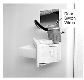
REASSEMBLY NOTE: Be sure to position either door switch with the straight side facing the front (see the top photo) before you press it into the opening.
