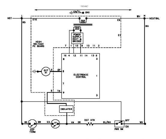
NOTE: When the power switch is off, the isolator sees line voltage. This keeps the electronic controller from signaling the evaporator fan motor or the compressor relay coils and also keeps the damper heater off.
