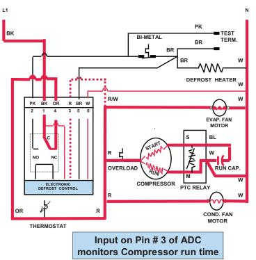
The ADC control supplies 120 VAC to the cooling circuit out of pin #4 The control monitors the compressor run time using an input signal on pin #3
