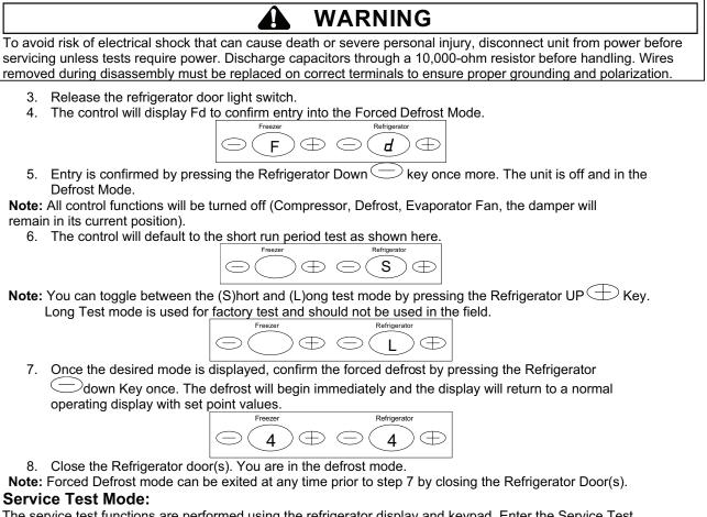
The service test functions are performed using the refrigerator display and keypad. Enter the Service Test Mode by performing the following sequence of events:
