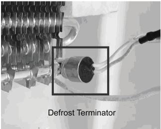
Some systems perform a defrost cycle based on elapsed time. A time is chosen as an interval between defrosts. Whenever the timer counts up the chosen amount of time, the system enters a defrost cycle. This type of system performs the defrost cycle without regard for the actual cooling demand on the sealed system.
