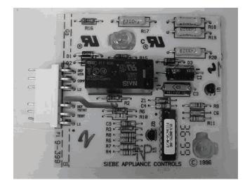
The theory behind an adaptive system is that an evaporator with a heavier frost load will take a longer time to reach the target defrosting temperature. An evaporator with a light frost load will reach the defrost temperature sooner. An ideal defrost time is chosen that should be reached with a frost load that is neither too light to warrant a defrost cycle nor too long to affect efficiency.
