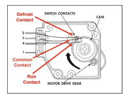
Although the contact numbers may differ from one timer to the next, all mechanical defrost timers work on the principle described above.
