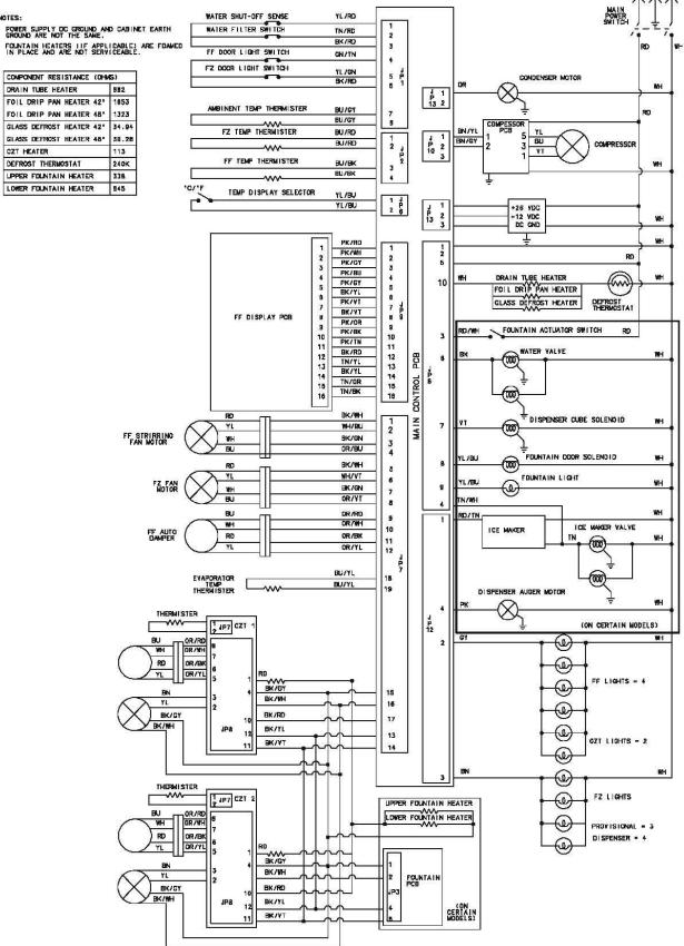
POWER SUPPLY DC CROUND AND CABINET EARTH GROUND ARE NOT THE SAME. FOUNTAIN HEATERS IIF APPLICABLE ARE FDAMED IN PLACE AND ARE NOT SERVICEABLE.
