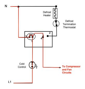
In the "cool" mode, contacts 1 and 4 of the timer are also made and this supplies power to the compressor and any fan motors that are in the circuit (evaporator and/or condenser).
