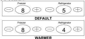
The last FZ Performance Offset value displayed before leaving test 8 will be saved when the refrigerator door(s) is closed.
