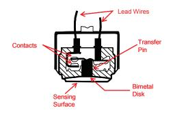
The defrost termination thermostat utilizes a bimetal disc to sense temperature. The disc is made of two dissimilar metals that expand at different rates. When exposed to temperature changes, the disc warps, making or breaking a set of electrical contacts.
