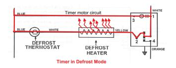
After the timer motor has run for the predetermined amount of time specified by the timer gears, the motor advances the internal cam into the defrost position. Contacts 1 to 4 open and contacts 1 to 2 close. This de-energizes the compressor and fans and energizes the defrost heater (assuming the defrost termination thermostat is closed).
