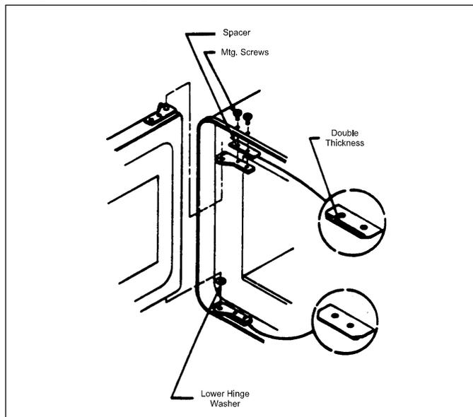
5. Install new door into lower hinge, leaving the door 1/2 way open. Place upper hinge and spacer on the top door pin. Spacer must be installed with the double thickness toward the oven front and toward the cavity overhang as shown. Install upper hinge mounting screws. Leave screws loose.
