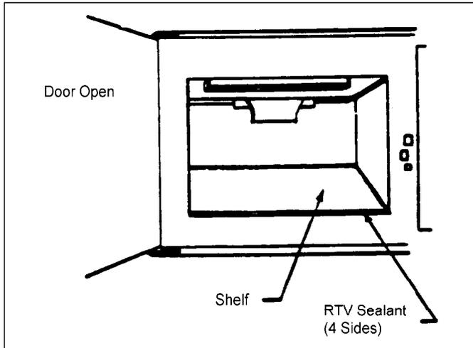
3. Insert a second screwdriver and slowly break the seal completely until the shelf is free.
