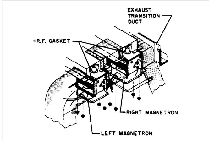
5. Remove four magnetron mounting nuts.
