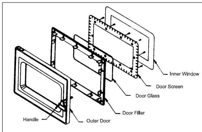
5. Install door on hinges as described under Door Assembly Replacement and Adjustment in this section.
