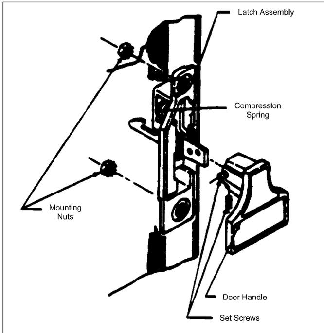
5. Install door latch assembly and reassemble door using new plastic inner window.
