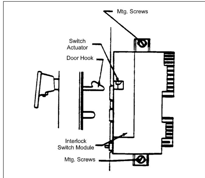
4. Retighten module mounting screws.
