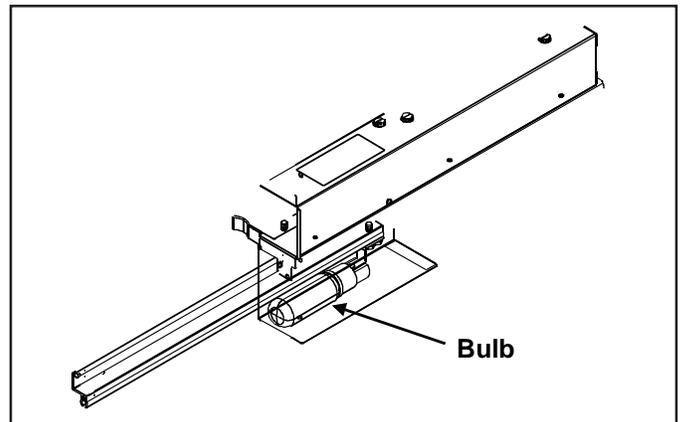
4. Remove bulb by turning counterclockwise, being careful not to burn fingers or break bulb.
