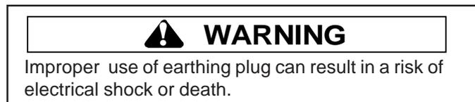
This equipment **MUST** be earthed. In the event of an electrical short circuit, earthing reduces risk of electric shock by providing an escape wire for electric current. This oven is equipped with a cord having earthing wire with a earthing plug. Plug must be plugged into an outlet that is properly installed and earthed. **DO NOT** use a two-prong adapter.
