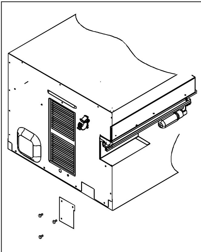
3. Slide rail out oven from oven cavity.
