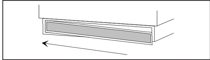
Remove splatter shield for easy cleaning.
