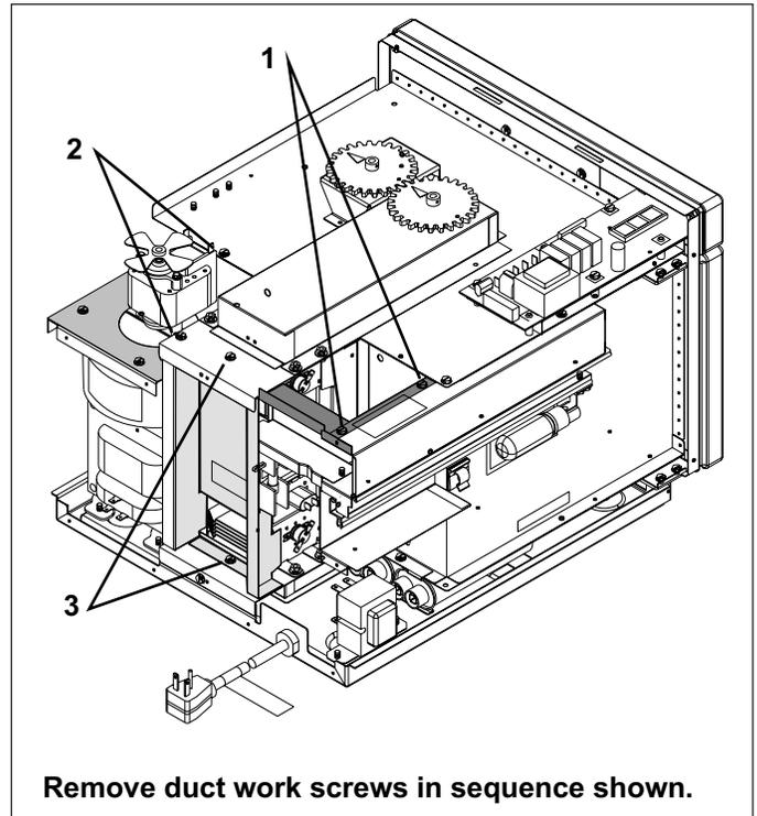
**Remove duct work screws in sequence shown.**
