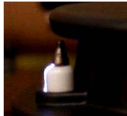
example: Spark jumps downwards respectively horizontal - not to burner cap – burner does not ignite
