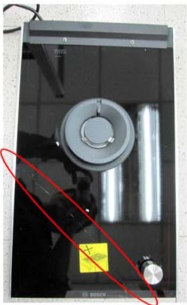
*Crack due to handling in factory*
