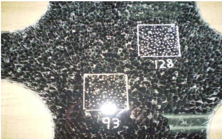
*Method of verification of the type of fracture*
