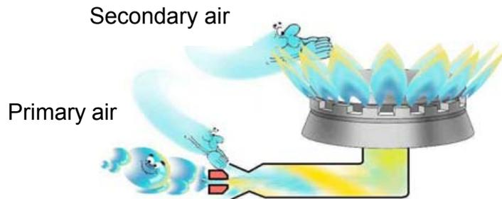
Clean, dry, undamaged and correctly assembled burner parts are essential for a stable, even flame and clean non-polluting combustion. Furthermore, the burning behaviour and flame aspect of the burners is defined mainly by:
