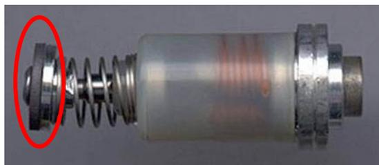
Silicon seal at plate of safety valve, could be missed or damaged
