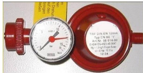
Very small leaks at the much bigger volume of secondary “low pressure” side lead to a more remarkable drop at the inlet “high pressure” side; i.e. a leak at the allowed limit of 40cm<sup>3</sup> at appliance would lead to a pressure drop at manometer of about 0,4 to 0,8 bar /h on 20°C propane ( which means 8 bar pressure at inlet, exact value of drop depends on volume of secondary side).
