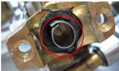
Torsion to manifold can occur at installation procedure, when there is tried turn the elbow without unscrewing the nut or when the nut is tightened again to the elbow without counter -keeping it with a second tool. This is also explained in installation manual with below graphics:
