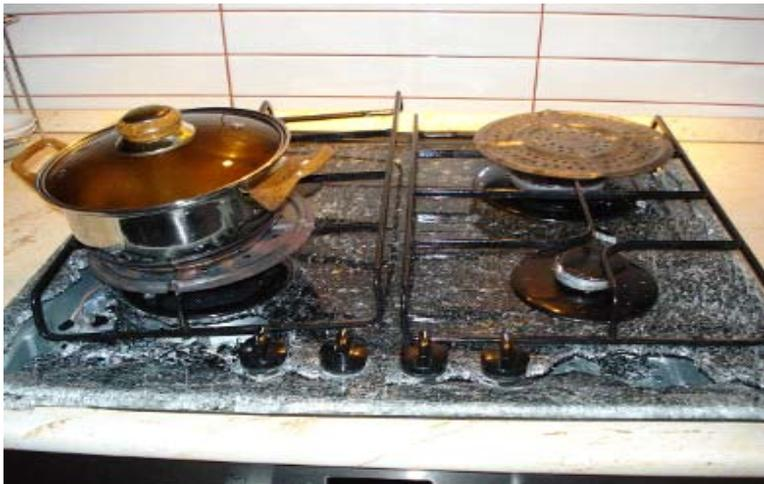
*Hob top broken due to the use of thermal diffusion plates*
