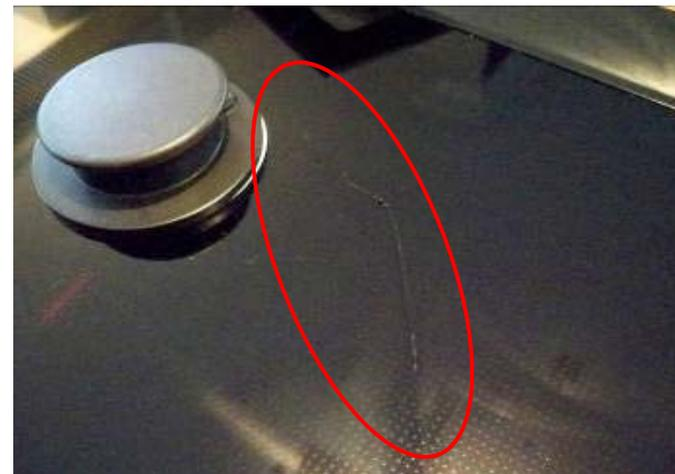
*Crack due to contact of the glass with metal edge component*
