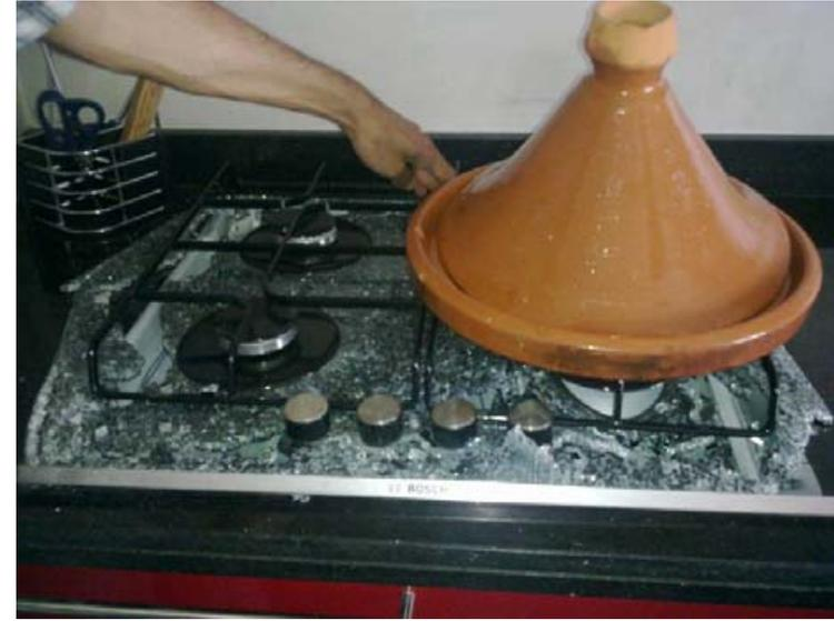
*Drip tray broken due to the use of a recipient of refractory material of large diameter*
