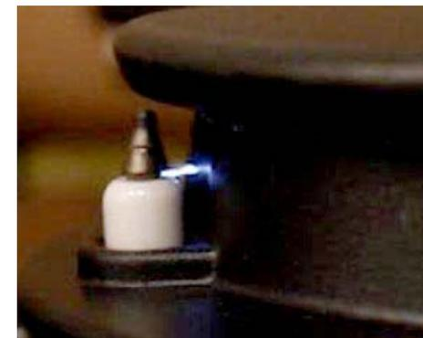
Example: spark jumps correct to burner cap – burner ignites
