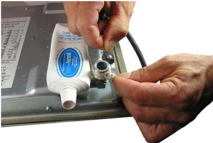
Example: elbow with conical thread (ISO 7) which has put on hemp and fermit for tightening
