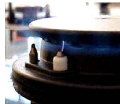
Hint: in principle all above consequences exists parallel, but in the real live a deviation in assembly from specified position will be visible in nearly all cases first at the ability to ignite burner.
