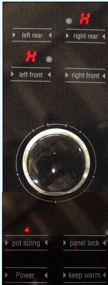
To select heating level, touch desired element, then twist knob.
