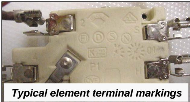
*For dual elements, the terminal #'s are also stamped on the metal element housing.*
