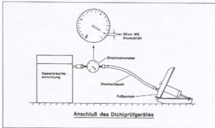
This gas-tightness testing appliance is available under Part Number 340034. It can be connected directly to ½" pipe (using 059155 sponge-rubber sealing plug).
