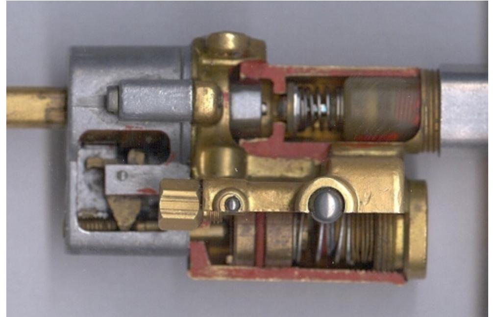
The set turning angle for the operating spindle (temperature preselection) tensions a counterpart against the valve disk by means of a spindle and push-rod system, thus influencing the volume of gas flow and, in the final analysis, the prevailing temperature in the oven.
