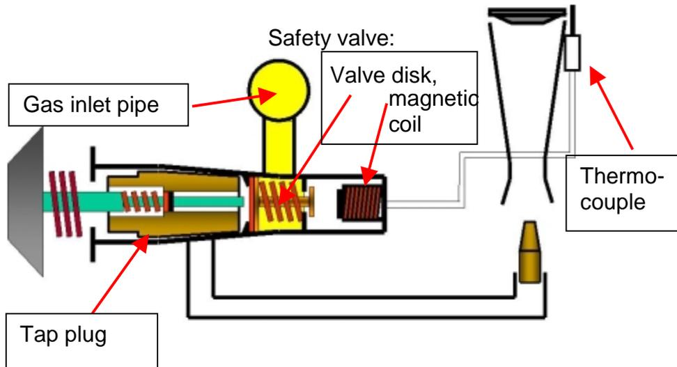
In the off position, the safety valve disk is pressed against the end-stop by the spring, thus closing off the flow of gas into the tap.
