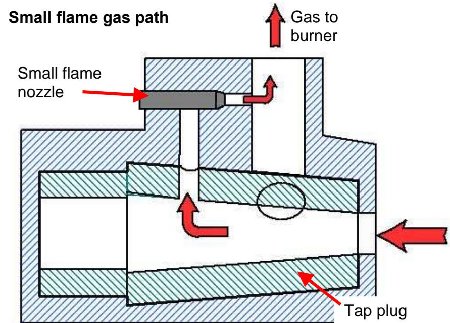
Each burner requires a minimum quantity of gas to ensure stable burning. (If this amount of gas is not supplied, the burner goes out, however when the design delivers excessive gas quantities for the low setting, customers tend to complain that "food is burned".)
