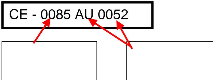
In some cases, this number is requested by installing companies or gas suppliers even before appliances are made available (these bodies can calculate technical specifications for gas appliances by referring to the Product Identification Number, thus permitting them to plan installations and networks).
