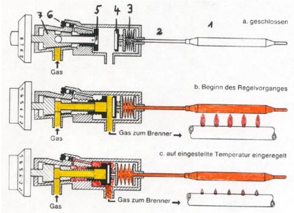
In cold state, the flow of gas through this valve disk is maximised, irrespective of the temperature setting. The maximum burner output channelled through is determined by a main nozzle located externally (in the oven burner). As the sensor heats up, the valve disk is pushed
