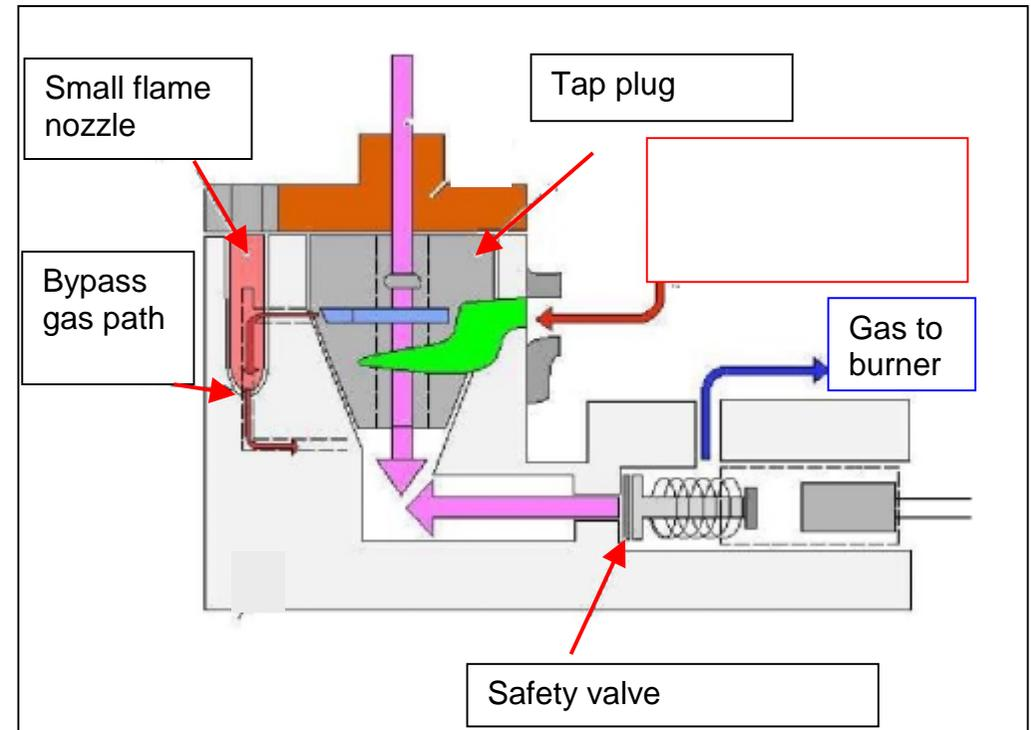
The function of the angle tap with thermal release is basically the same as described above (straight-through gas tap).
