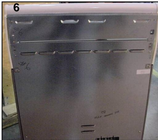
Remove the screws which hold the 2 rear panels and disconnect the ground screw from the maintop support
