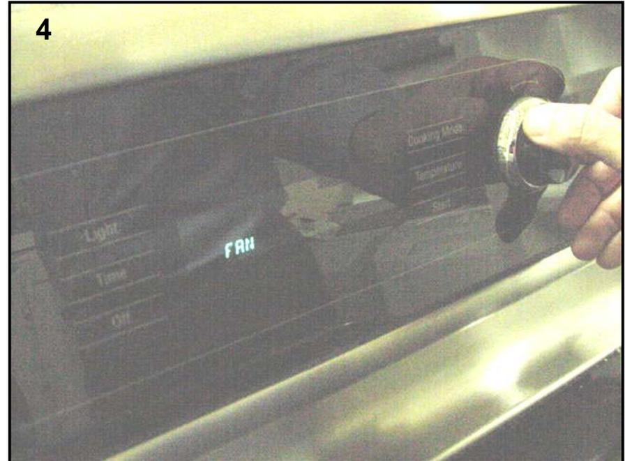
**Note:** During all functions the maximum oven temperature is 200F, if reached the display shows TOO HOT and any function in operation stops, except the Off ( which allows exit from the program). The test can be resumed once the temperature falls below 200F.
