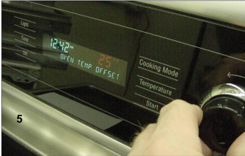
Using the control knob scroll through the temperature options. The temperature ranges from -25F to + 25F. Select the number of degrees that the temperature needs to be changed by and touch [Start]. Display will show **SELECT FUNCTION**, touch [Off] to complete the change.
