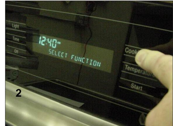
Using control knob, scroll through menu until **OVEN TEMP OFFSET** appears. Touch [Start] and a number will appear in the temperature window. If the oven has never been calibrated before it will be 0F.
