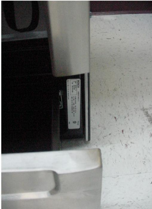
The first 4 digits of the FD number designate the year/month the model was produced. For instance, FD number beginning with 86 were built in 2006; 87 = 2007; 88 = 2008, etc.
