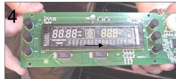
Remove upper rear access panel, remove connector from board, remove the 6 screws holding the board. Reassemble new board in reverse order after checking the board configuration. See next page for instructions.
