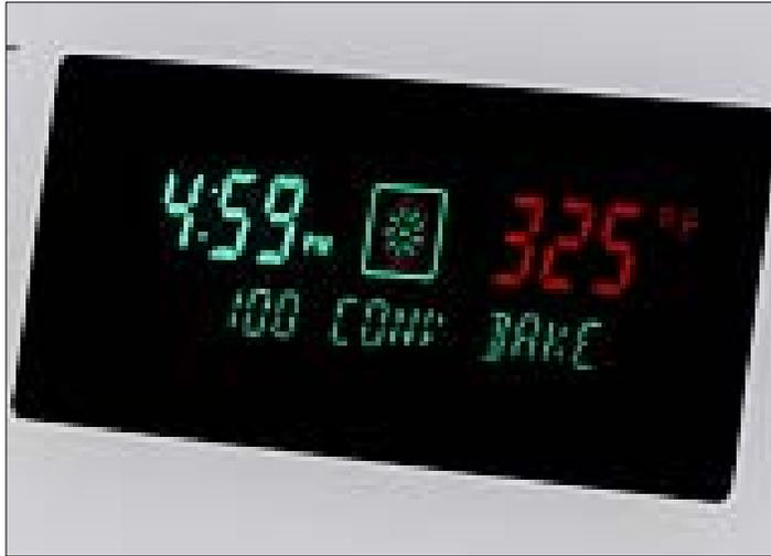
1. Touch [Bake] and set temperature at the control. The relay board receives input and checks resistance of sensor. If heat is required the following relays will close: K3 & K4 for the bake element and K1 & K2 for the broil element.
