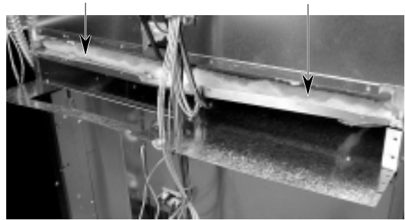
Bend Flange Down To Access Bake Element
