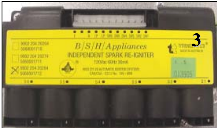
Spark module is powered by Spark switch activating only that channel
