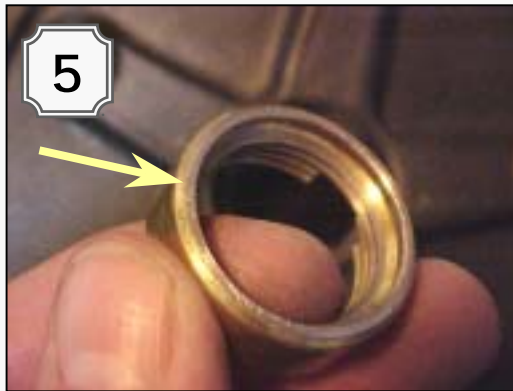
Check nut -- sand if necessary to insure a good ground
