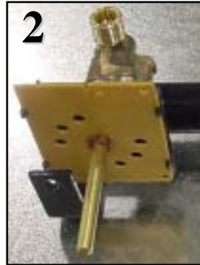
Rotation of knob opens control valve & changes resistance at potentiometer, changing voltage
