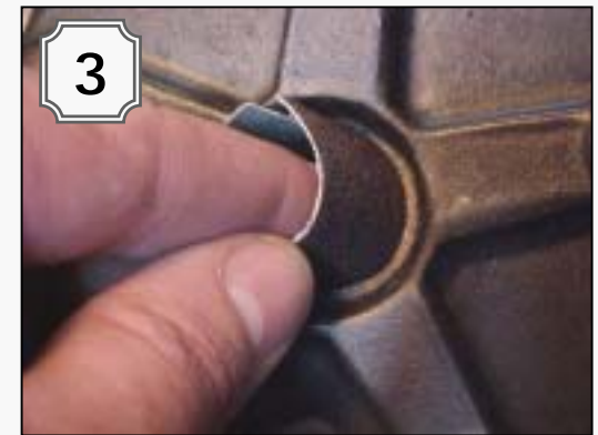
Using emery cloth, sand mating area to remove coating
