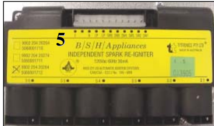
Spark module is powered by simmer controller activating only that channel
