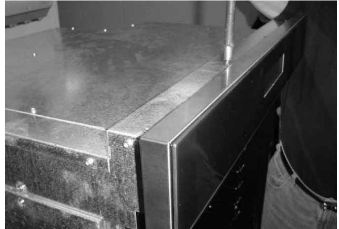
Screws on Top of Control Panel
