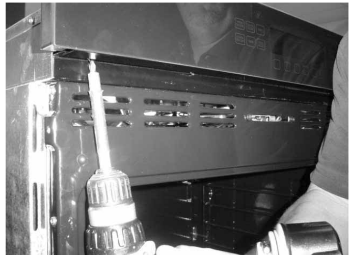
Screws on Bottom of Control Panel
