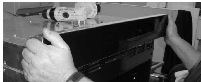
Control Panel Removal
