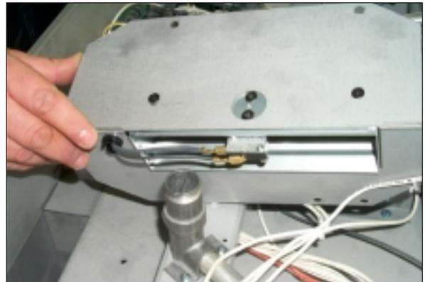
1. Remove 2 nuts w/lock washers from case back (stud is welded)
