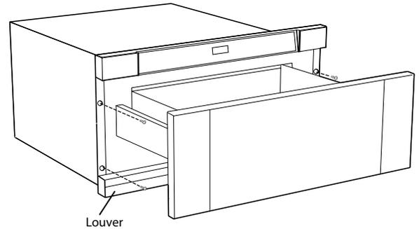
2. Open the Drawer to access the 4 mounting screws holding the unit on to the wall or cabinet opening. **(Fig 1)**.
