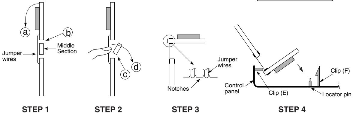
**POSITIVE LOCK® CONNECTOR (NO-CASE TYPE) REMOVAL**
