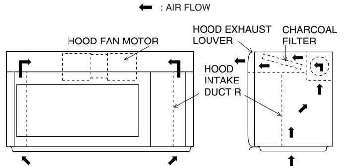
**VENTILATION METHODS HOT AIR EXHAUST**
