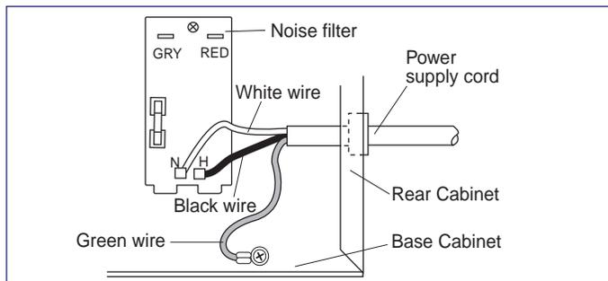
**Figure 4-3. Power Cord Connections**
