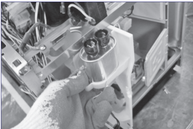
Figure 4-4. High Voltage Capacitor
