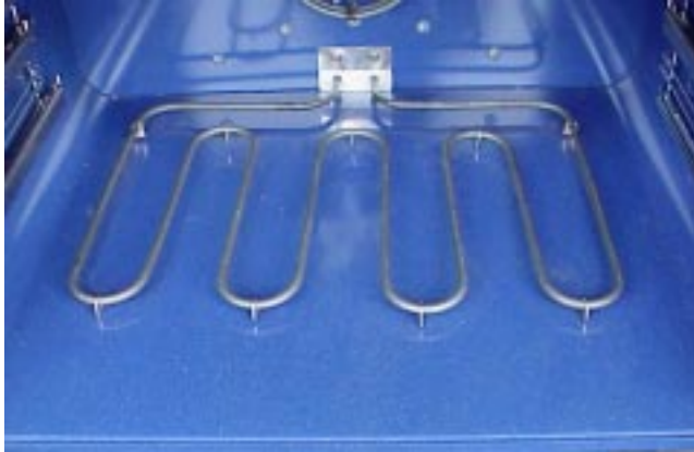
broil element mounted to the top of the oven,
