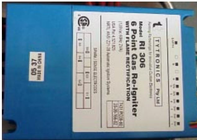
gas igniter/re-igniter module
