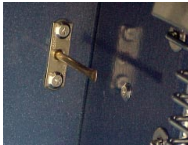
oven sensor mounted to the rear wall of the oven,
