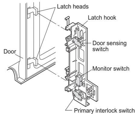
Figure C-1. Latch Switch Adjustments
