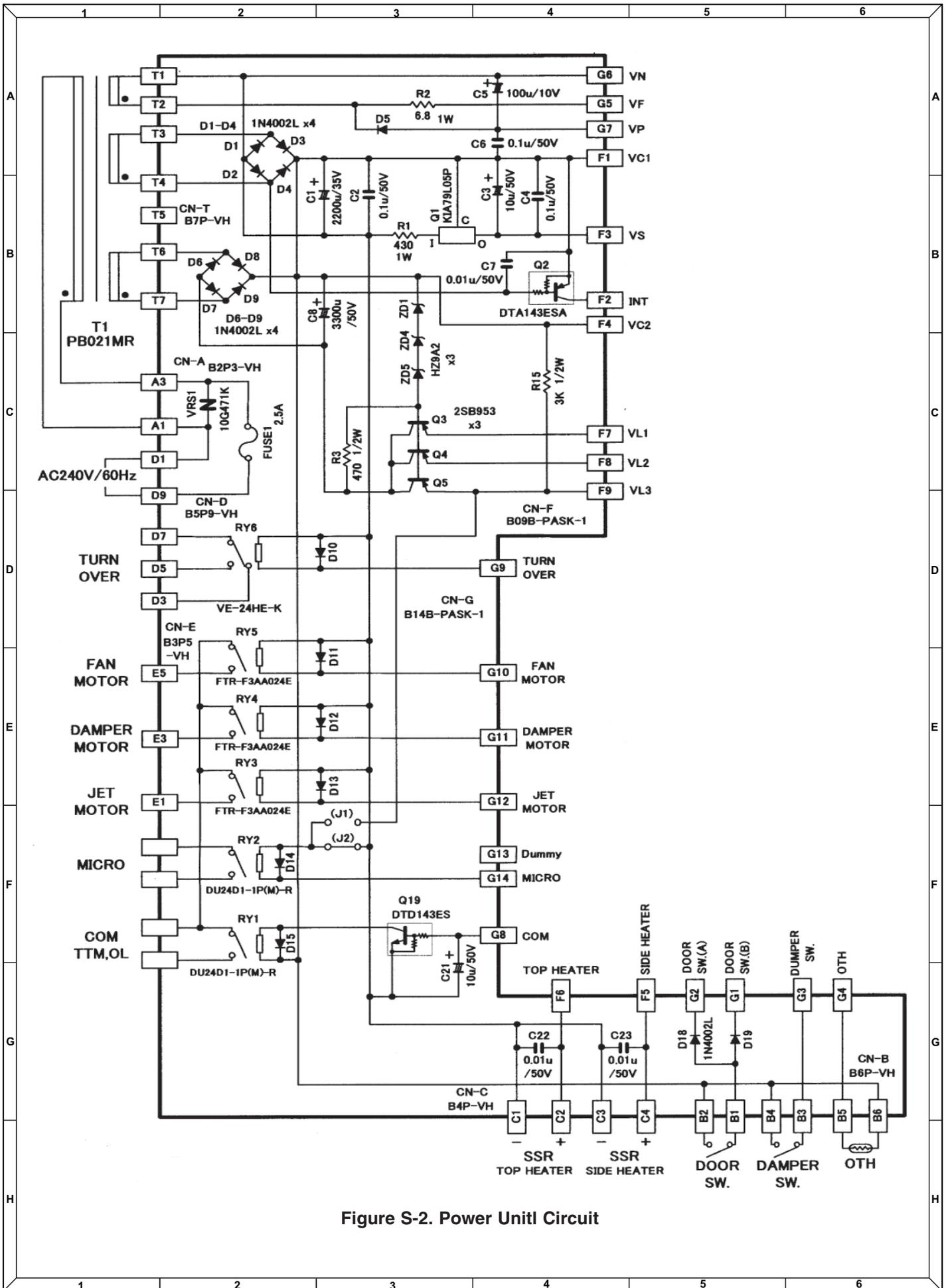
Figure S-2. Power Unitl Circuit
