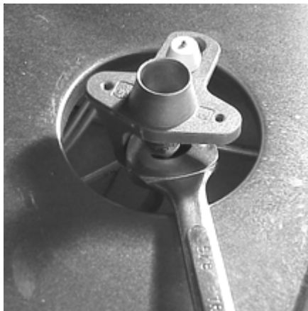
Removing burner base
