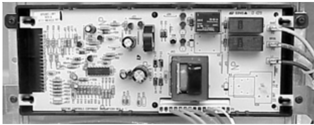
Back view of electronic oven control
