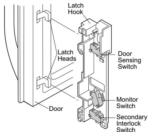
Figure C-1. Latch Switch Adjustments
