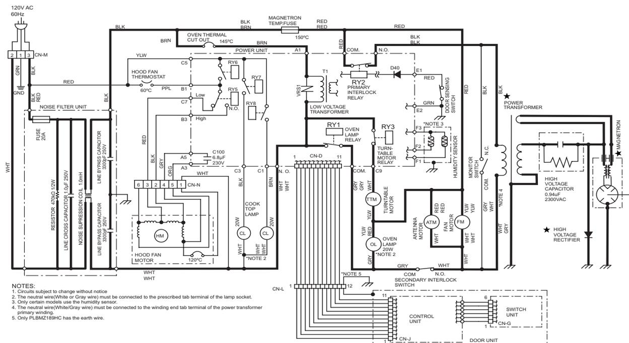
Figure O-2. Oven Schematic-Cooking Condition
