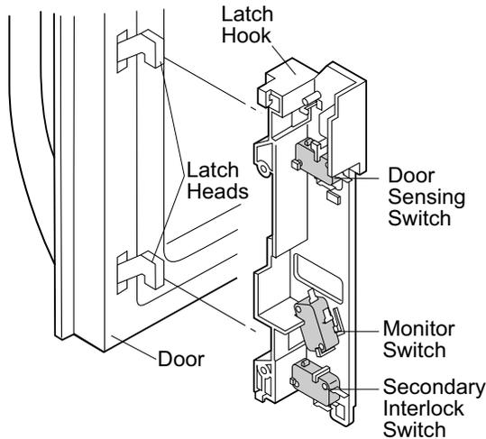
Figure D-1. Door Open Mechanism.
