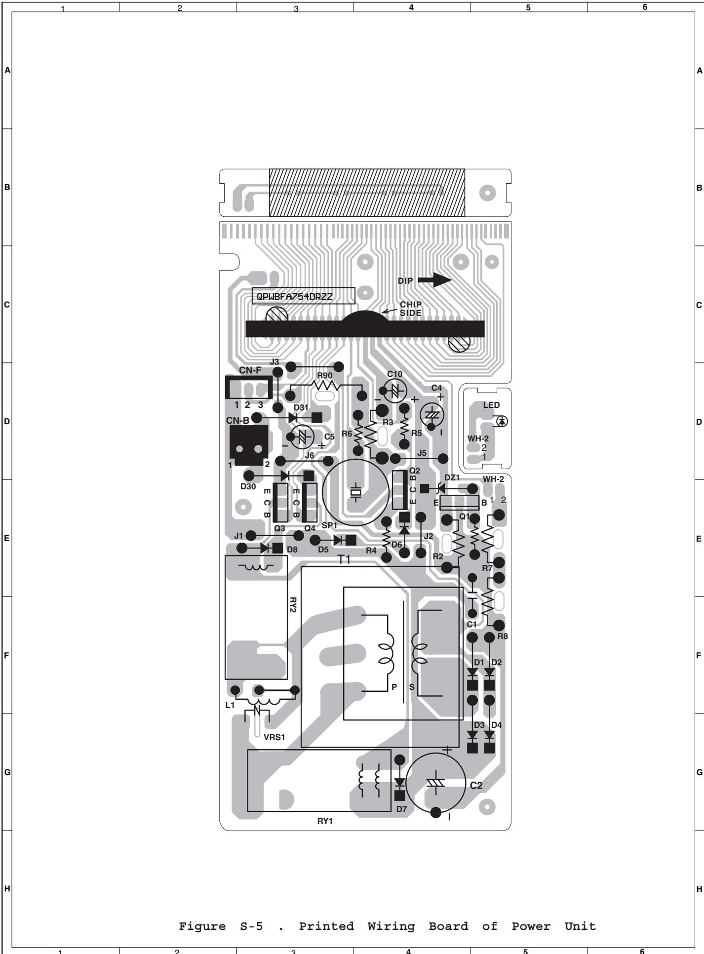
Figure S-5 . Printed Wiring Board of Power Unit
