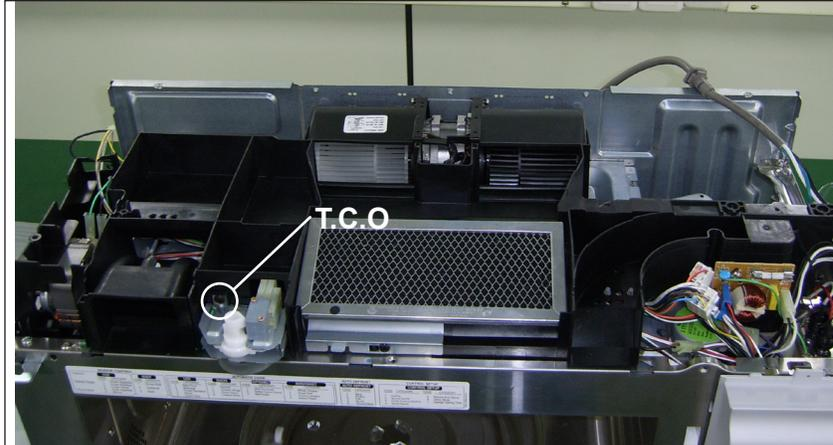
2. Loft up the exhaust duct from the cavity.
