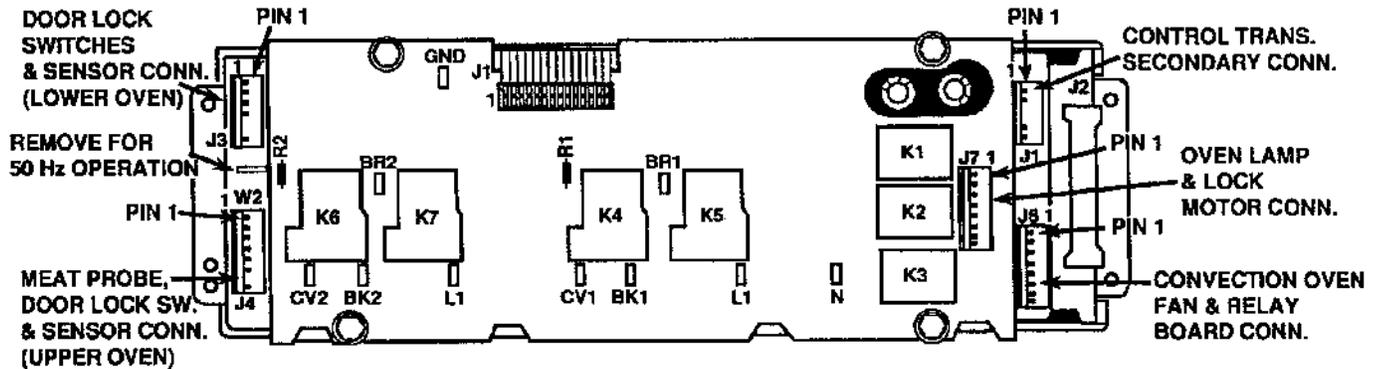
**NOTE:** ON CONVECTION MODELS - Convection Connector (J6) must be properly aligned (Pin 1 to Pin 1) to avoid damage to control.
