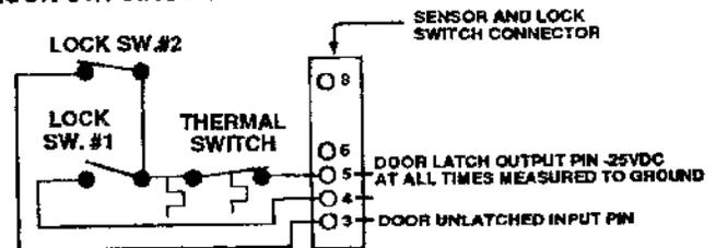
**NOTE:** Lower Oven lock circuit same as upper oven except for the two thermal switches.
