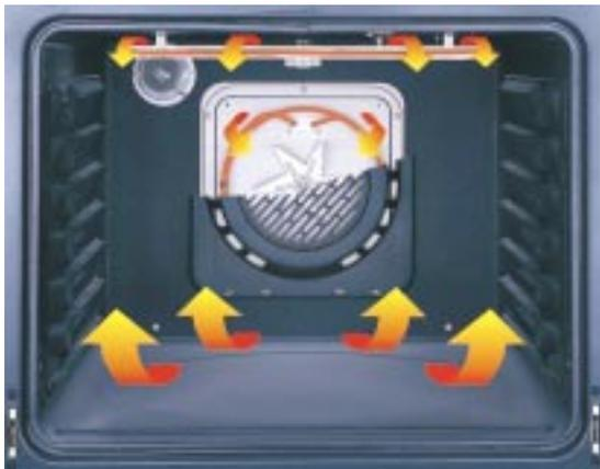
GE Convection ranges use the European or "true" convection system. The difference between "us and them" is a third dual loop heating element that surrounds the convection fan in the back wall of the oven. The convection fan at the rear of the oven, gently circulates heated air evenly throughout the entire oven cavity, under and around the food. The moving air penetrates foods faster than stationary air.
