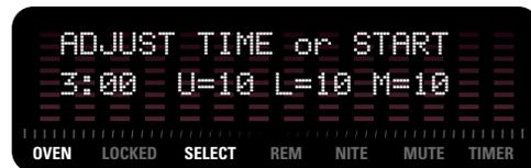
Notice that the display shows power levels of 10 for each cooking component. During this test you will be operating the oven with no load. For this reason, it will be necessary to **adjust the microwave power level to zero (M=00)**. To do this, press the power level button on the control panel. Leave the upper and lower power levels at 10 (U=10 L=10), and adjust the microwave to zero (M=00).
