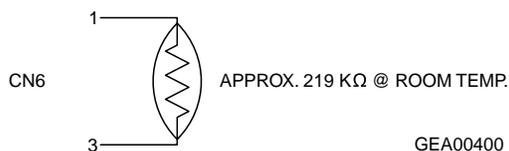
The oven cavity thermistor has a negative temperature coefficient. In other words, as the temperature of the thermistor probe increases, the resistance of the thermistor decreases. This
