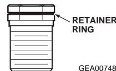
3. Using a 7-mm or 9/32-in. nut driver, remove the natural gas orifice from each burner and save. These may be accessed through the hole in the main top.
