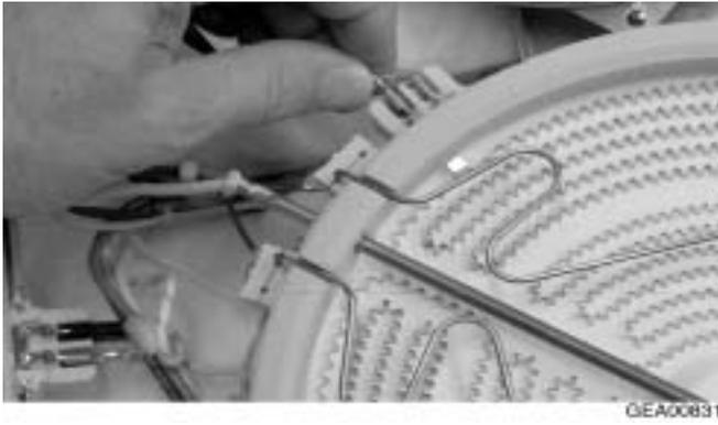
4. Remove the electrical connectors from the heater.
