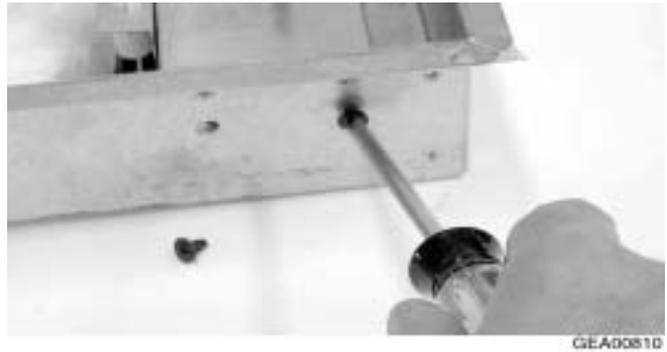
2. Remove 4 screws from the switch mounting bracket (2 from each end).
