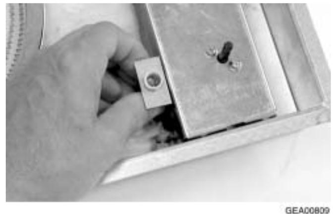
2. Compress the ON light wings, as shown, and pull down to remove from the bracket.
