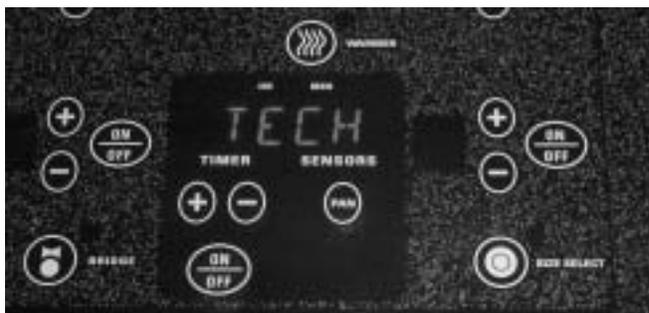
To clear the F-code register, enter Technician Mode. While the timer display flashes *TECH MODE*, simultaneously press the BRIDGE and WARMER keys. The timer display will display *DONE* and the F-codes will be permanently deleted from the register.
