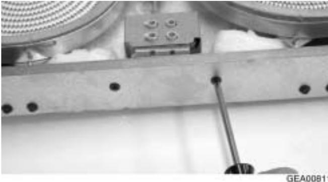
4. Remove 4 screws from the switch mounting bracket (2 from each end) and remove the red wire from the switch for the left rear burner.
