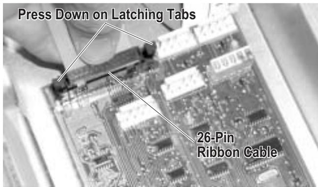
3. Disconnect the 26-pin ribbon cable from the logic board by pressing down on the latching tabs of the header.
