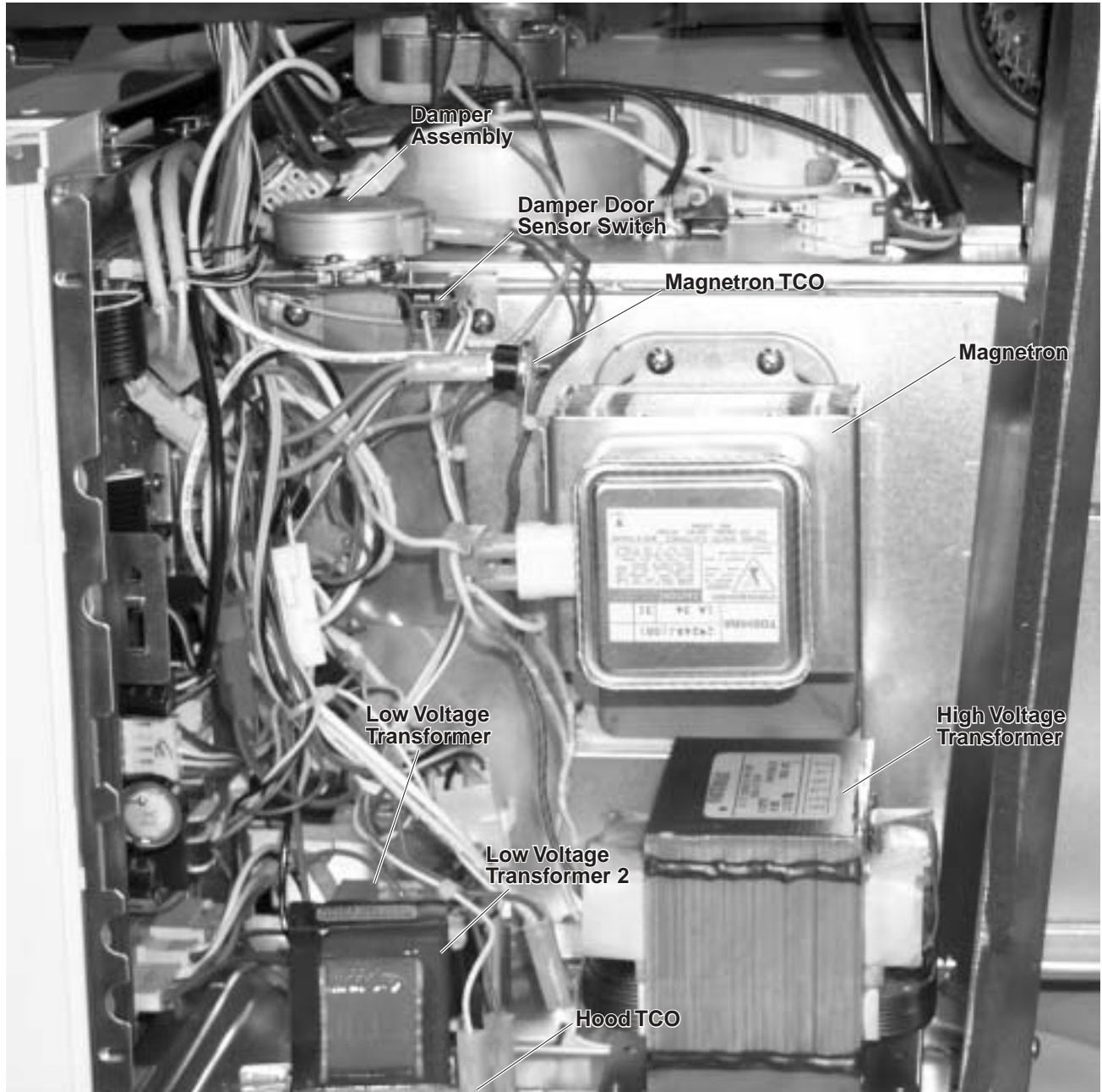
Figure 4 - High Voltage Compartment
