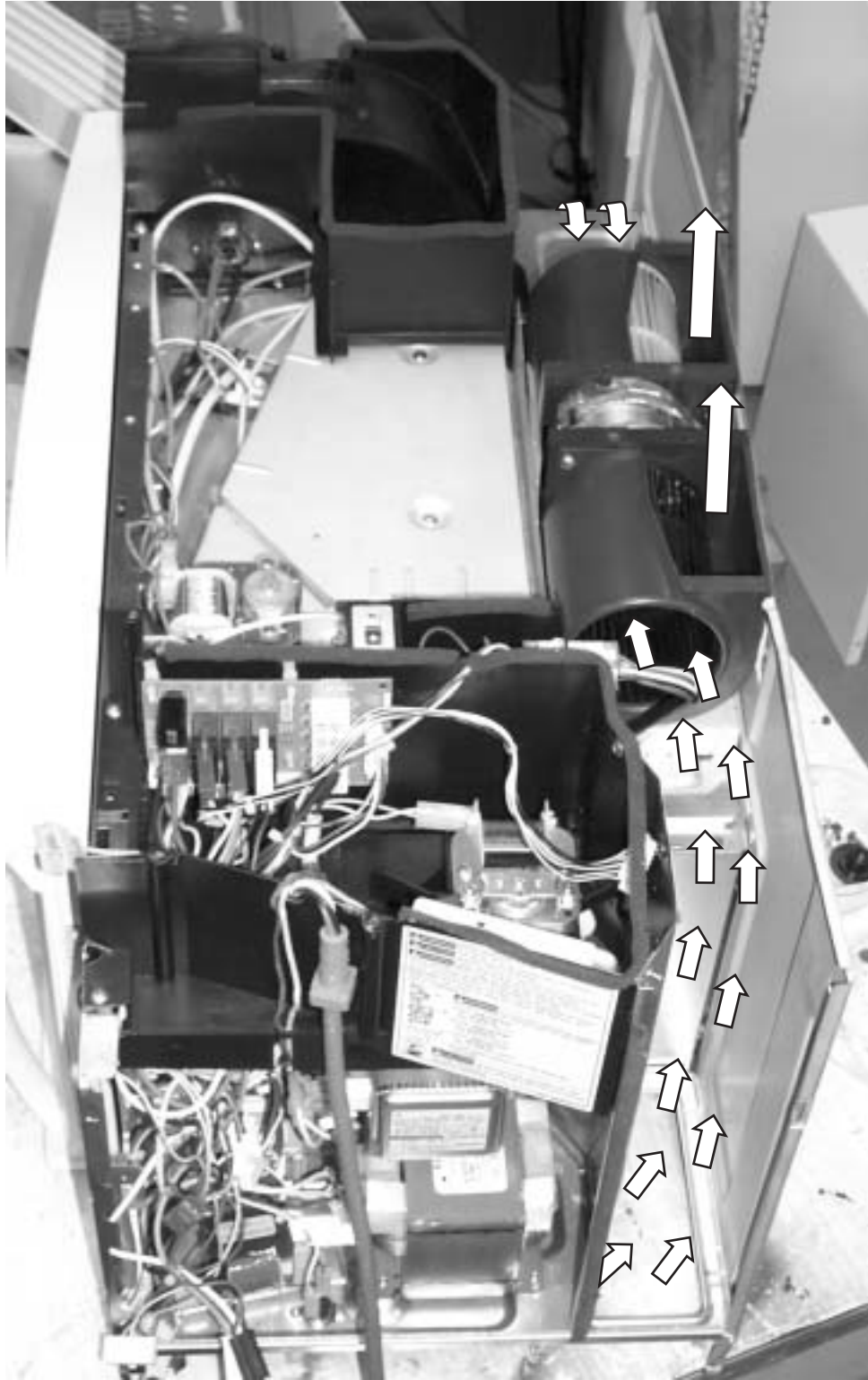
Figure 3 - Vent Fan Airflow
