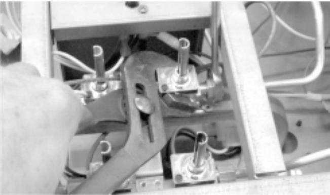
3. Remove the 1/2-in. nut on the gas line to the valve and remove the gas line.
