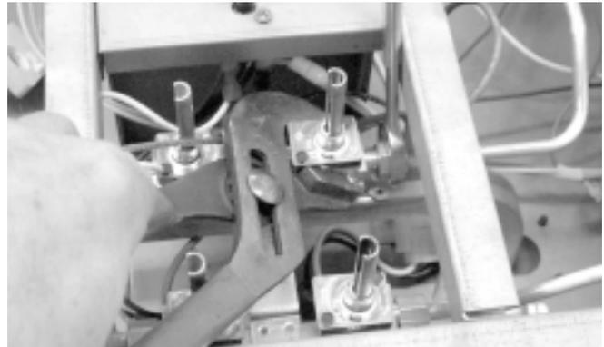
3. Remove the 1/2-in. nuts (4) on the gas lines to the valves and remove the gas lines.
