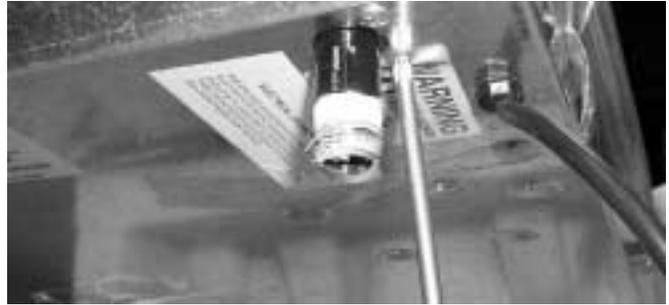
6. Remove two 5/16-in. nuts and the valve.
