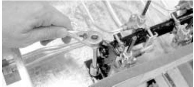
7. To reinstall the valve, make sure the valve is seated on the manifold and the valve stem is vertical.
