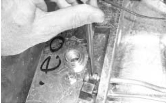
3. Remove the 5/8-in. nut on the jet holder and remove the jet holder.
