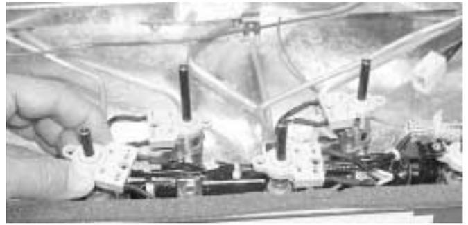
**Note:** When replacing the switch, replace the entire harness with colors in same positions. The bottom of the switch is molded to conform to the top of the valve for a locked-in fit. Reconnect both ground wires and replace wire ties.
