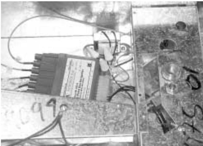
3. Remove 2 green ground wire connectors and 1 wire nut connection to the transformer.
