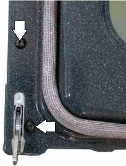
3. Remove the four ¼-in. hex-head screws that attach the glass and side brackets (glass closest to the outer door glass) to the inner door.
