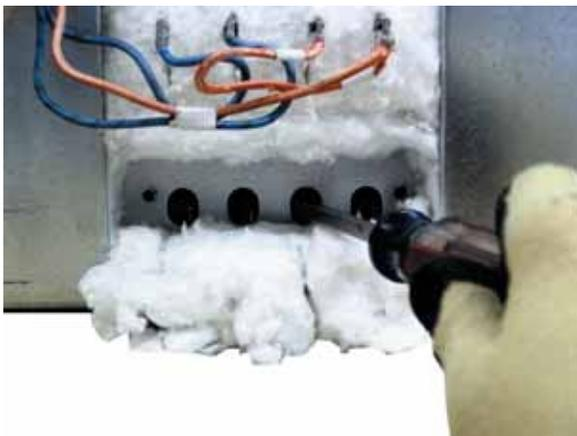
8. Grasp and pull the element out from the left side of the oven.
