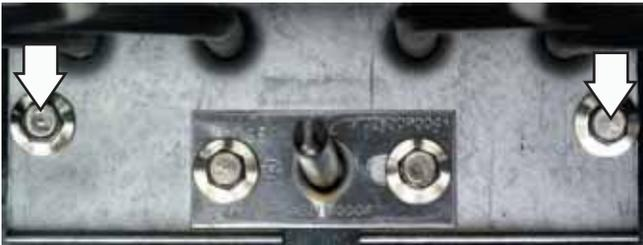
4. Carefully pull the sensor and sensor wiring harness from the oven liner.
