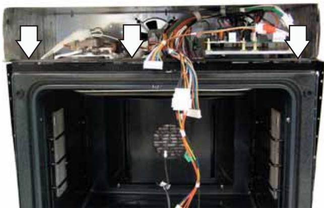
4. Carefully reach into the control compartment and slide the capacitor out of the restraining clamp.
