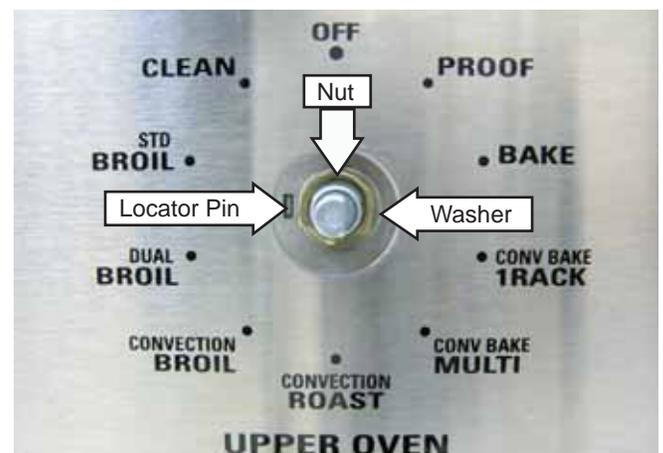
**Note:** To ensure proper alignment, position encoder locator pin in control panel slot before tightening nut.
