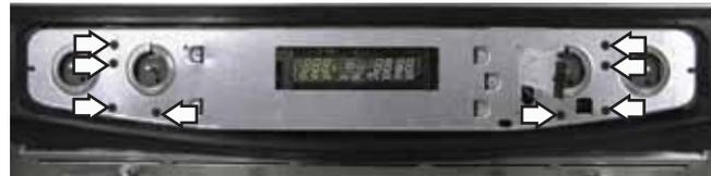
5. Position a protective surface over the top of the range and place the ERC in the service position.
