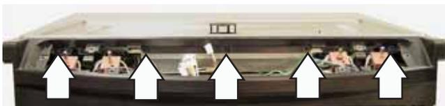
4. Remove each single burner igniter. (See *Surface Burner Igniters*.)
