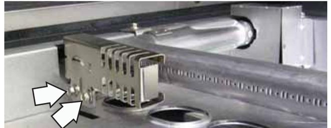
8. Gently pull the igniter wiring and harness through the bake burner box.
