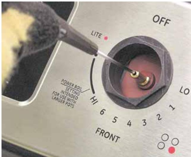
2. Find the valve bypass screw through the access hole located to the lower right side of the valve.
