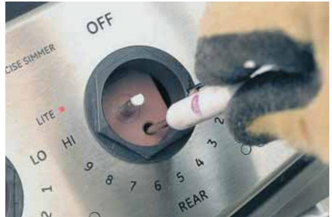
4. If the flame appears too low or unstable, adjust the valve bypass screw slowly (turn counterclockwise—CCW) until a stable flame exists for each burner. Remember, two other burners must be turned on to medium.
