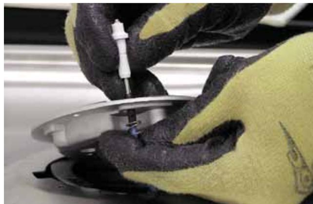
**Note:** When installing, replace the inner two T-20 Torx center screws first. Partially tighten the T-15 Torx screw opposite the igniter and align the remaining screw holes. Replace the remaining 2 screws.
