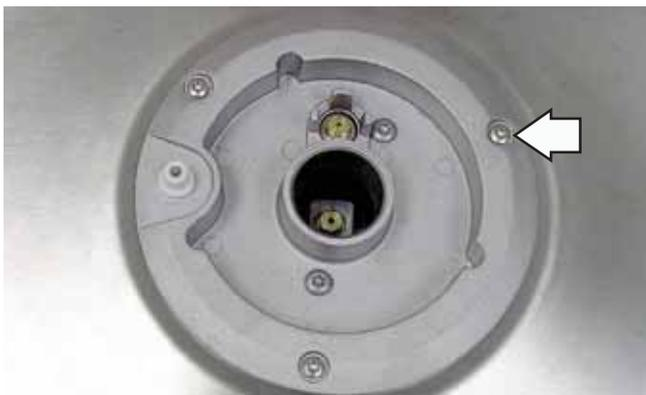
3. Remove the outer two T-15 and the inner two T-20 Torx screws, then lift the dual burner base to access the igniter.
