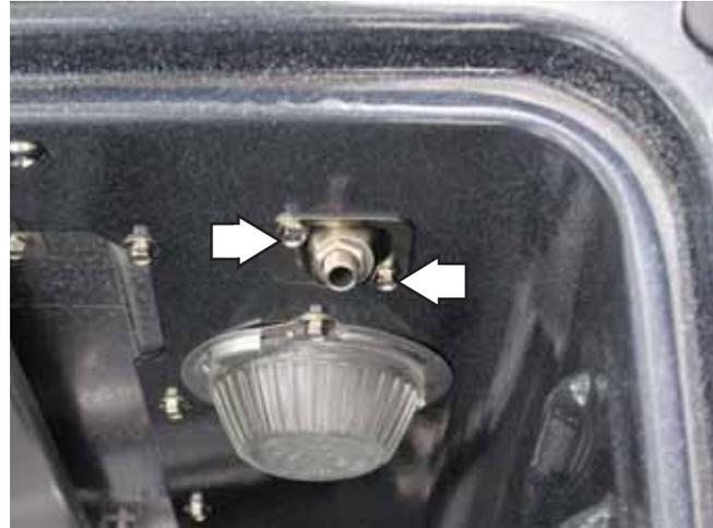
The outlet and wiring can then be pulled down from the oven wall approximately 1½ inches.
