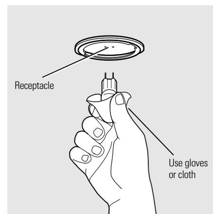
To replace a light bulb, use a new 130-volt halogen bulb, not to exceed 50 watts.
