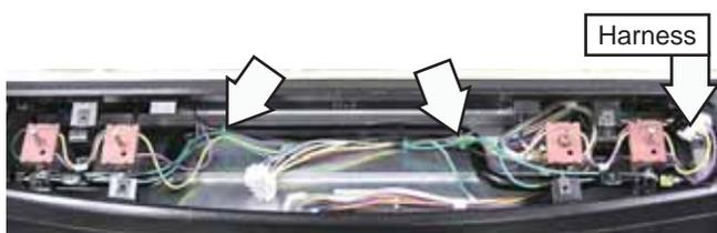
4. Lift each igniter switch from the burner valve stem and remove the igniter switch assembly.
