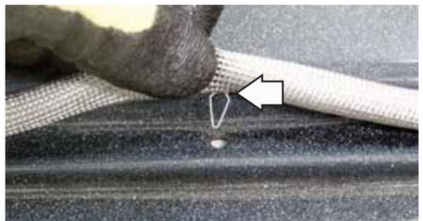
When installing the door gasket, it is helpful to fold the gasket in half and locate the center clip. Insert the clip at the top of the door and work your way around the door.
