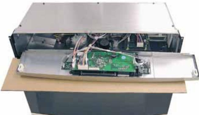
4. Mark and disconnect connectors from the lock assembly.
