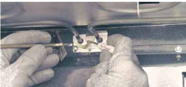
**Note:** When reinstalling the sensor, use a small flat-blade screwdriver to push and guide the sensor wire harness into the oven liner.
