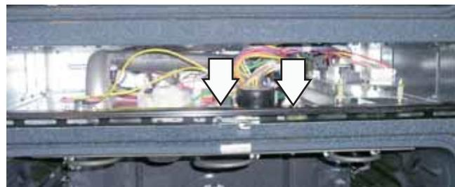
4. Mark and disconnect connectors from the lock assembly.
