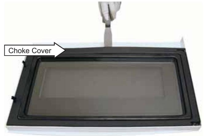
3. Remove the 5 Phillips-head screws from the choke (3 on top, 1 each on bottom and latch side).
