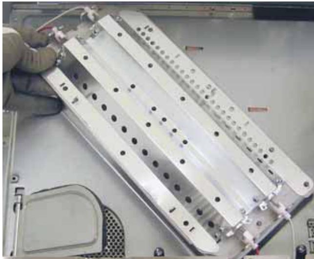
**Bottom View of Halogen Heater Assembly**
