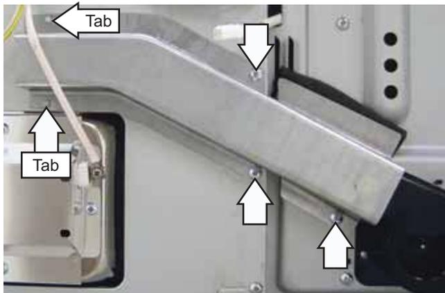
5. Remove the 3 Phillips-head screws that attach the blower outlet to the bottom of the Lower Cooling Motor.
