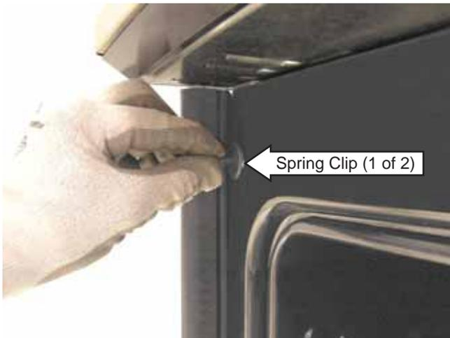
3. Insert a small flat-blade screwdriver on 1 of 2 spring clips and depress the spring clip while pulling the switch from the door frame.
