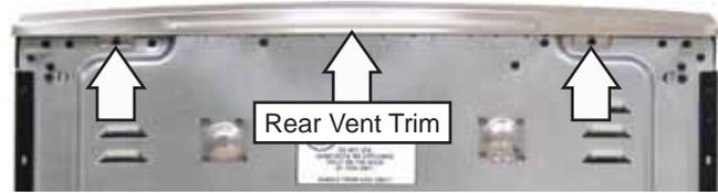
5. Remove the five 1/4-in. hex-head screws (3 at the rear and 2 on top) that attach the rear vent to the range. Lift and remove the rear vent.
