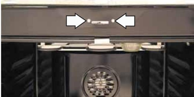
5. Pull the oven door lock assembly toward the rear of the range.
