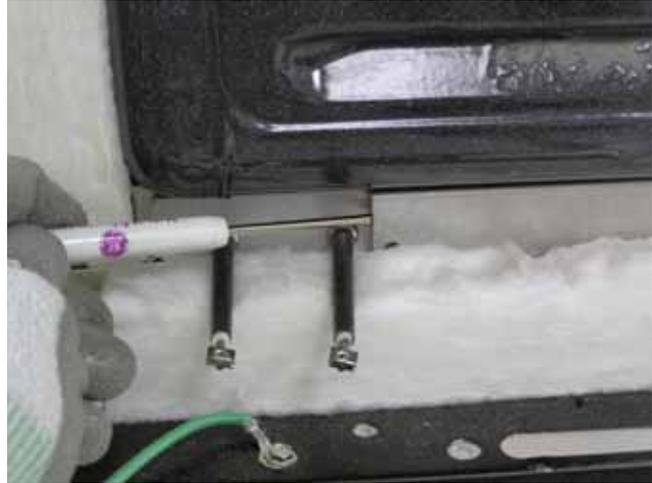
21. Pull the retainer to the left, and disengage the tab from the slot in the element tray.
