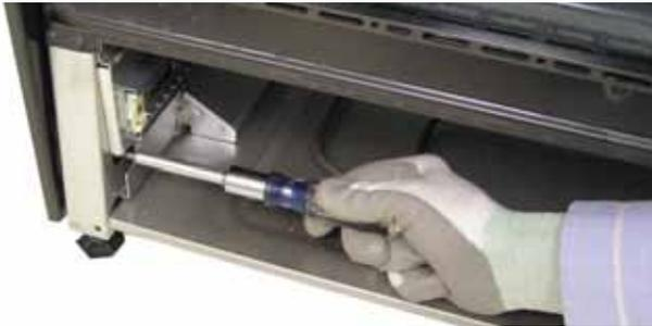
7. Remove the five 1/4-in. hex-head screws (3 at the rear and 2 on top) that attach the rear vent to the range. Lift and remove the rear vent.
