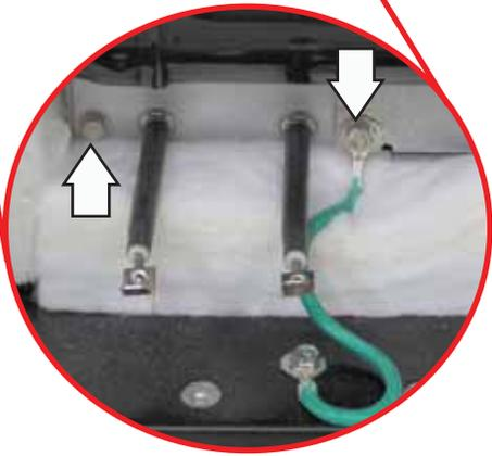
20. Using a small flat blade screwdriver, pry the left side of the retainer away from the element.
