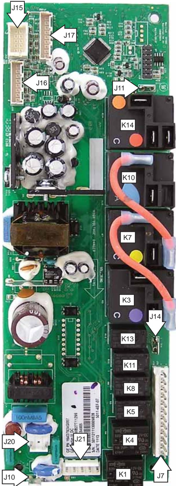
J7 - Door Lock Motor, Cooling Fan, Jumper Wire K8 to K1, Warming Drawer Element, Neutral, Oven Light, Convection Fan Motor Direction
