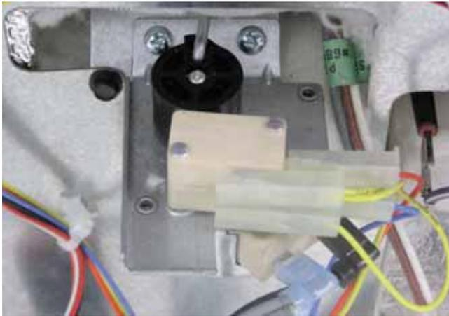
To remove the upper oven door lock assembly:
