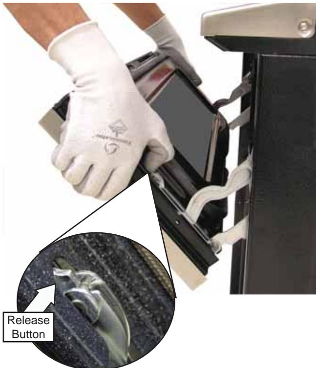
5. Lift the door up until it is clear of the door hinges.
