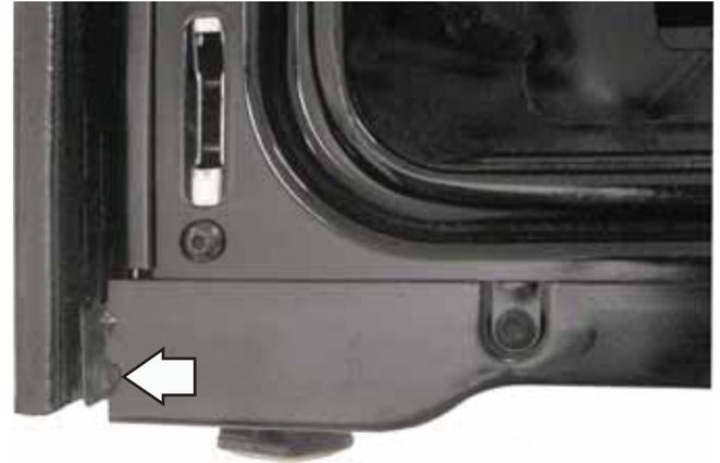
3. Remove the six 1/4-in hex-head screws from the top front of the control panel support.
