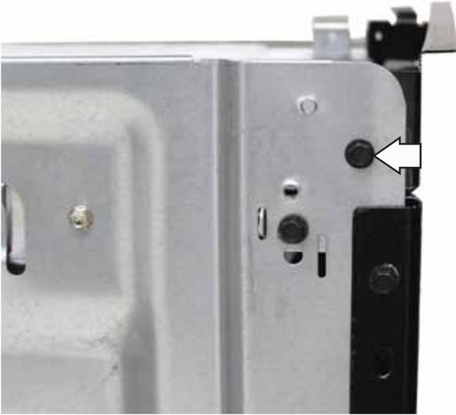
11. Carefully lift the left side of the control panel support, slide the extension brace forward and remove the extension brace from the range.
