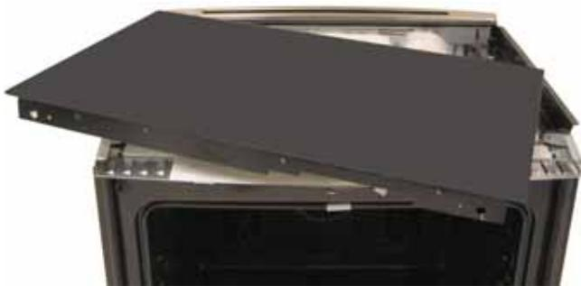
4. Remove the two 1/4-in. hex-head screws that attach the rear vent trim to the range. Lift and remove the rear vent trim.
