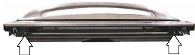
4. Remove the T-15 Torx screw from each side of the outer door panel.
