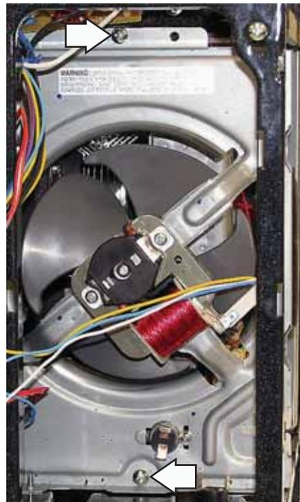
8. Move the cooling fan frame out thru the right side of the microwave oven.
