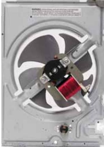
9. Grasp the hub of the cooling fan blade and pull the cooling fan blade off the motor shaft.
