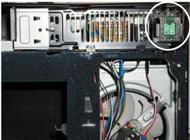
The power saver battery snaps into the plastic holder, which, in turn, snaps onto the grille.
