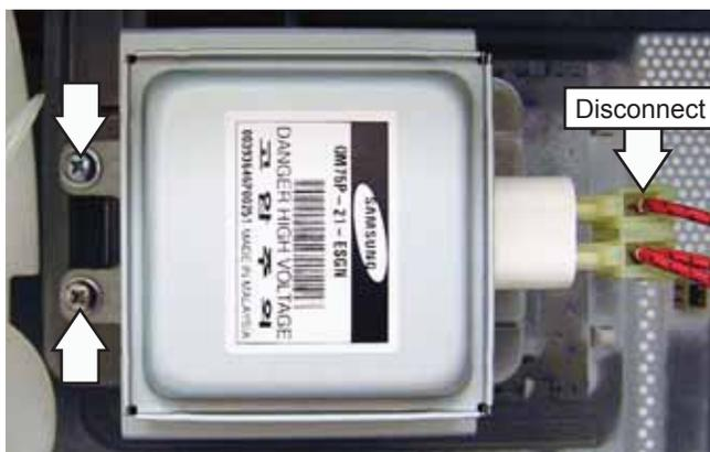
4. Disconnect wiring to the magnetron TCO.
