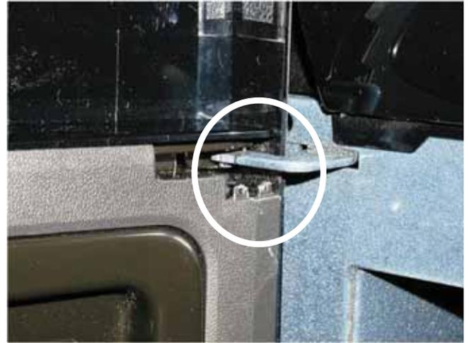
Lift door to disengage upper and lower door hinge the pins from the hinge arms.
