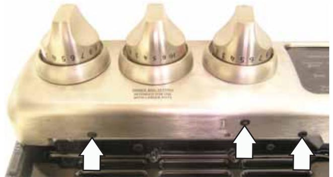
3. Pull the 6 knobs off the control panel.
