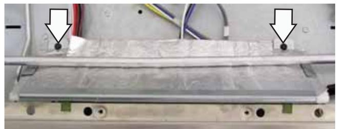
6. Pull the fiber barrier out of the control panel.
