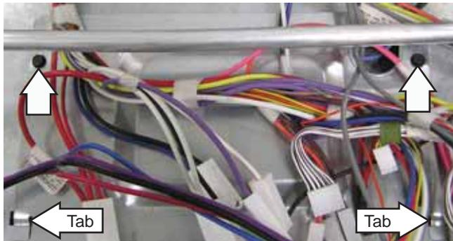
5. Remove the two 1/4-in. hex-head screws holding the door lock assembly to the frame.
