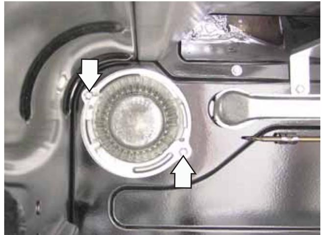
Pull the light assembly away from the oven liner to access and disconnect the 2 wires.
