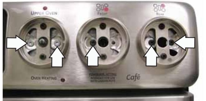
5. Remove the two 1/4-in. hex-head screws and the heat shield.
