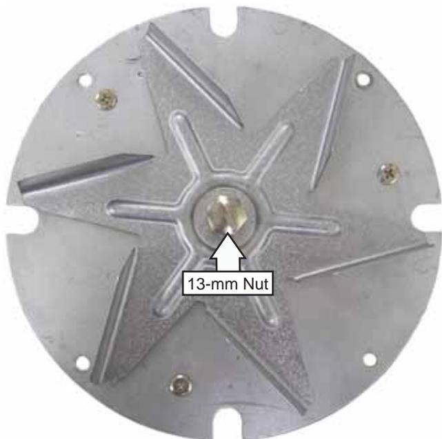
**Note:** The fan blade is attached to the D-shaped motor shaft with a left-hand thread.
