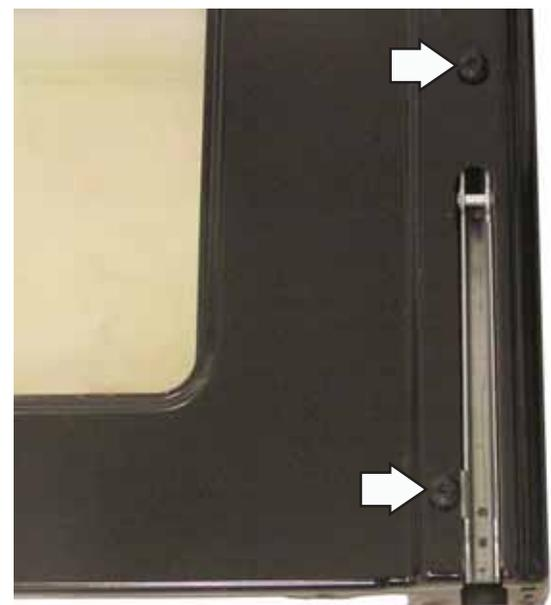
3. Remove the 10 Phillips-head screws and the heat barrier from the inner door.
