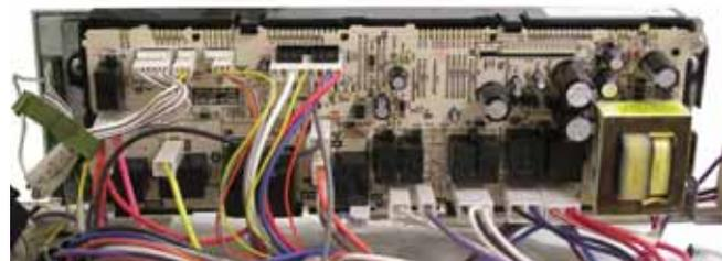
13. Remove the 4 Phillips-head screws from the control board bracket.
