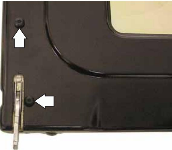
4. Remove the 10 Phillips-head screws and the heat barrier from the inner door panel.
