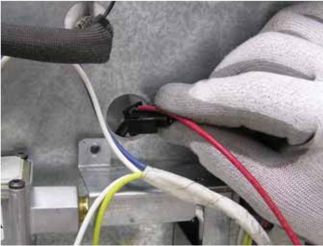
14. Carefully pull the igniter and part of the retrieval wire thru the opening at the bottom right corner of the upper oven.
