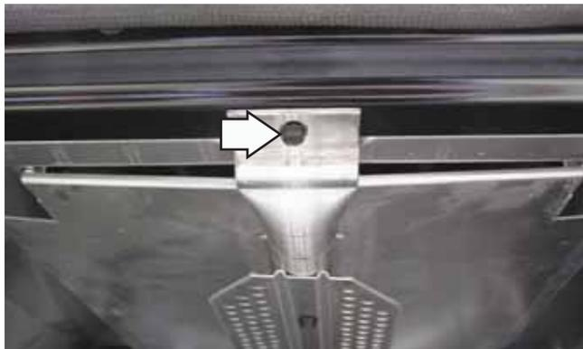
3. Remove the two 1/4-in. hex-head screws that attach the glow bar igniter to the side of the broil burner.
