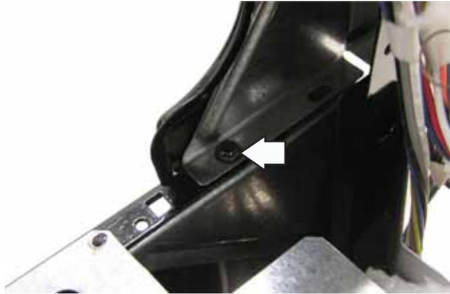
6. Remove 4 Phillips-head screws from the top of the side panel.
