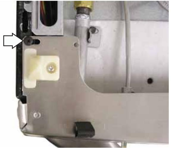
4. Remove the 4 Phillips-head screws from the bottom of the manifold panel (2 on each side).
