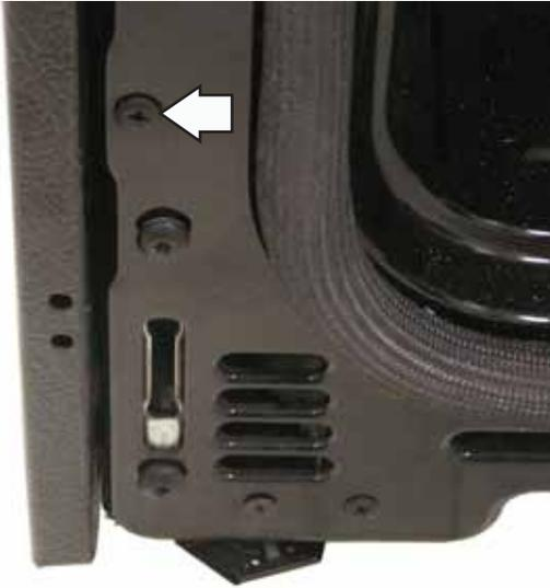
7. On Profile and GE models, remove the extra 1/4-in. hex-head screw holding the side panel to the rear touch panel and ERC bracket.
