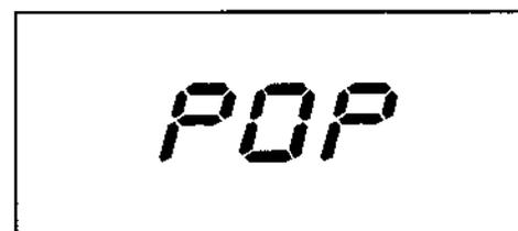
4. The popcorn sensor automatically calculates the cooking time. After the popcorn sensor detects steam, the oven signals and displays remaining cooking time needed.
