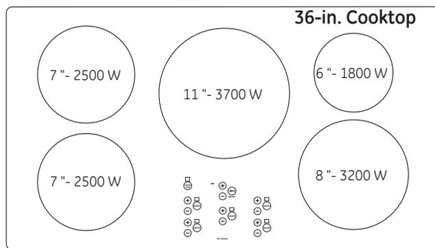
Generator board maximum output is 3700W. When using an element on high and a second element sharing the same generator board is then operated, the second element will receive priority. For example, if the first element was using 3700W when the second element was turned on, power on the first element will be reduced to a lower setting.
