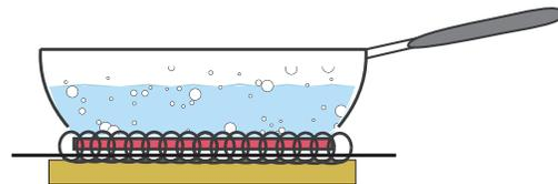
By heating only the bottom of the pan, the surrounding surface remains cooler than with traditional cooktops.
