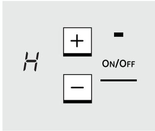
"H" indicates that the Boost power level has been selected for rapid cooking and boiling.
