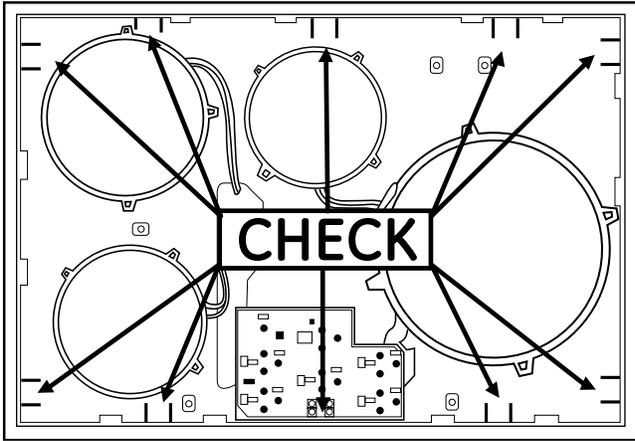
In the following illustrations, the heat shield is out of alignment due to an excessive flat-bottom drop of the cooktop. A large flat blade screwdriver can be inserted in the gap on the left-side of the tab.
