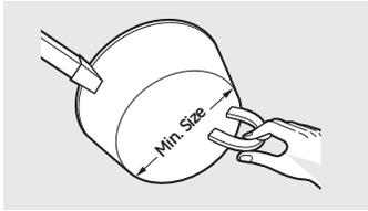
Use the minimum size pan for the element. The pan material is correct if a magnet sticks to the bottom.
