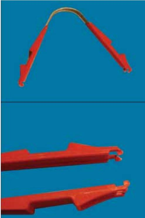
**Correct way:** Use side-to-side motion to remove the LINbus connector.
