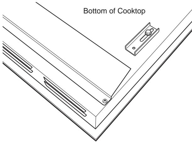
**Note:** In the following step a baffle is not installed if cooktop is installed over an oven.
