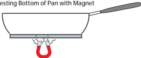
When the proper type of pan is placed over an energized induction coil, a field of magnetic waves will cause the bottom of the pan to heat.
