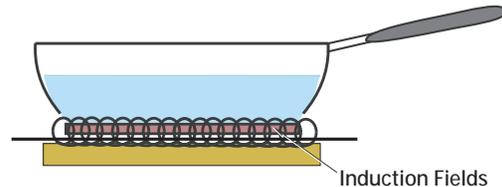
The contents of the pan are therefore heated more quickly than they would be if heated by a gas flame or a traditional radiant heating element.
