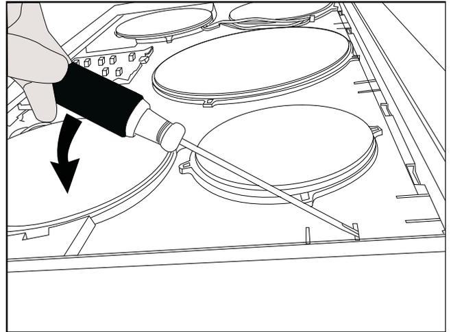
Inspect all tab-to-heat shield alignment areas. Repeat this alignment procedure on all tabs, if necessary.
