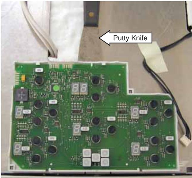
**Note:** If one or more functions do not work and no apparent damage is present, the cause can be an excessive flat-bottom drop of the packaged unit during shipping/handling. The force of the drop can position the heat shield out of proper alignment to the heat shield mounting tabs. This would cause improper spacing between the underside of the glass top and the capacitive switches on the module, rendering the switches inoperative.
