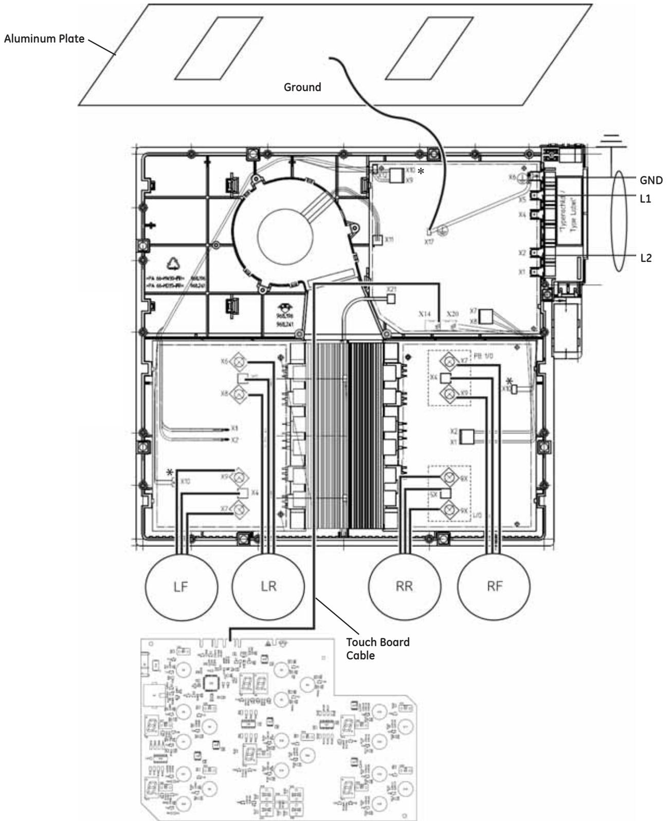
**Caution:** \*A special tool is required when removing the connections (marked with an \*) from the circuit boards. (See *LINbus Connectors*.) Damage to the circuit boards or wiring harnesses may occur without utilizing the special tool.
