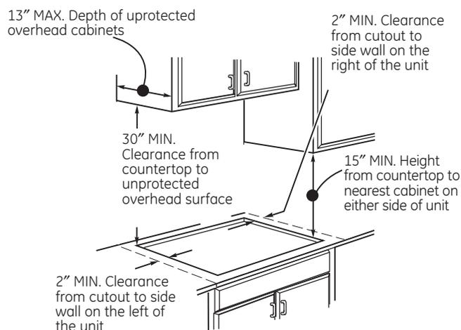
If a 30-in. clearance between the cooking surface and overhead combustible materials or metal cabinets cannot be maintained, a minimum clearance of 24-in. is required and the underside of the cabinets above the cooktop must be protected with not less than 1/4-in. insulating millboard covered with sheet metal not less than 0.0122-in. thick.
