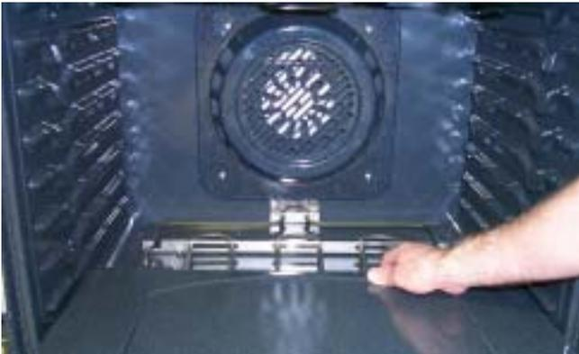
4. Remove the 2 hex-head screws that hold the element to the rear oven wall.
