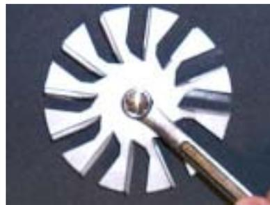
4. Remove the fan blade and washer from the fan motor shaft.
