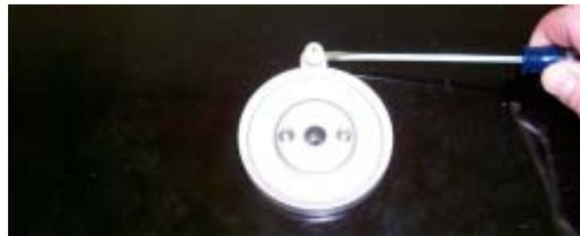
3. Unplug the wire from the back of the spark igniter.
