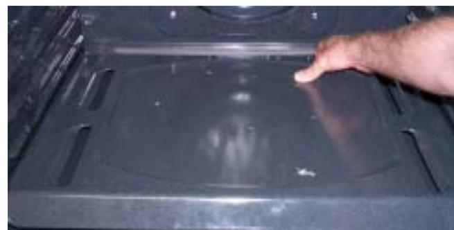
3. Remove the 4 screws that hold the burner baffle in place.
