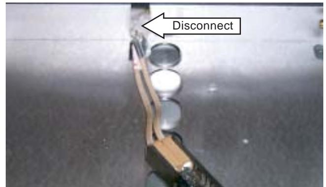
6. Remove the glow-bar igniter from the oven.
