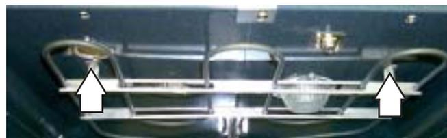
5. Carefully pull the broil element forward to access the wiring connections.
